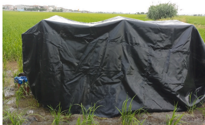
Fig. 2. Imaging under controlled light conditions (CLC) covering stereo video camera platform rails: artificial light was generated within the imaging space from a LED source with an illuminance of 460 lx ( \text{cd sr m}^{-2} ), approx.
