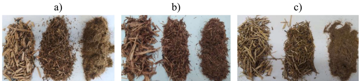
Fig. 4. Fractions of a) C. ladanifer , b) J. communis and c) R. officinalis after the sieving and blowing process.
