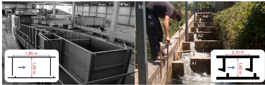
Fig. 2. Fish passage experiments. Studied fishways and geometrical characteristics. a) Lab experiments. b) Field experiments.
