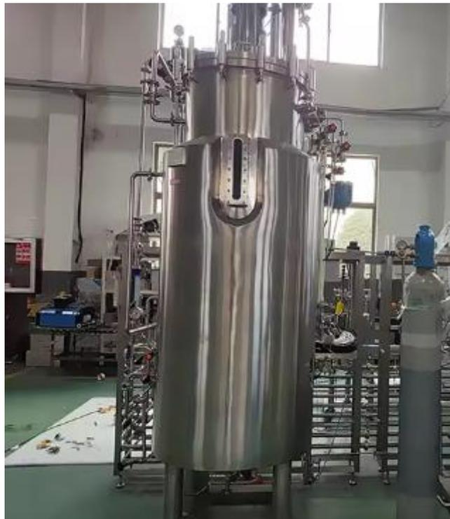
Figura 7: Biorreactor de SFS
