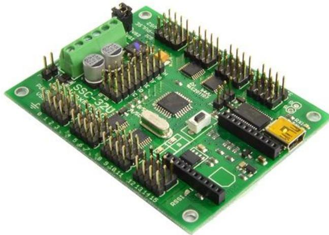
*Figura 19. Lynxmotion SSC-32U Servo Controller. Fuente [19]*
