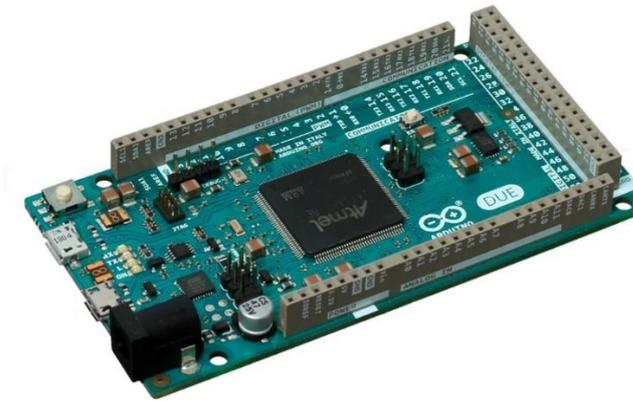
Figura 14. Arduino DUE. Fuente [14]
