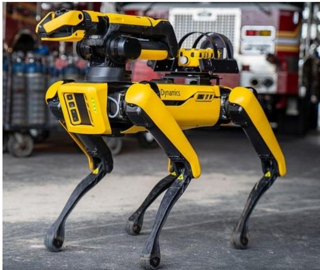
Figura 2. Robot Spot. Fuente [2]
