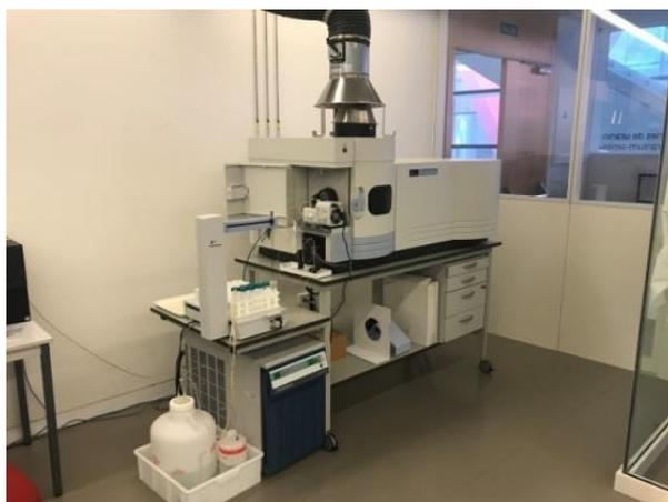
**Figure 14.** ICP-OES at CENIEH.
