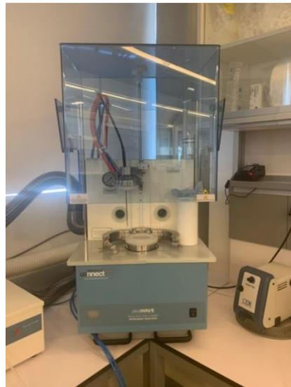
**Figure 11.** ultraWave Single reaction chamber microwave digestion at CENIEH laboratory
