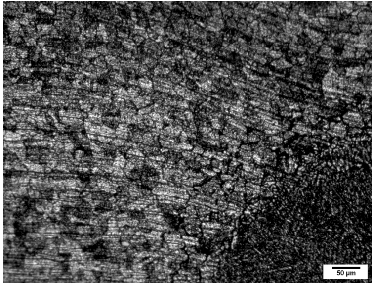
Fig. 4. Optical micrograph that shows the base metal and the zone adjacent to the weld nugget (specimen No. 6). Micrograph taken after DLEPR test.
