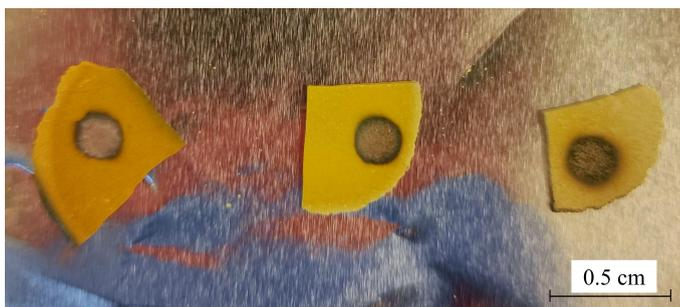
Figure 14: Pieces of the pellets (Figure 13) after the deposition of the gold coating using a shadow mask.
