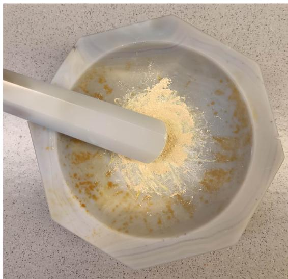
Figure 11: Mix of the composites in powder form, in a mortar and pestle.
