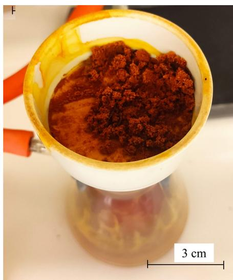
Figure 8: Photograph of a filtering flask, funnel, filtering paper and the dark red crystalline product.
