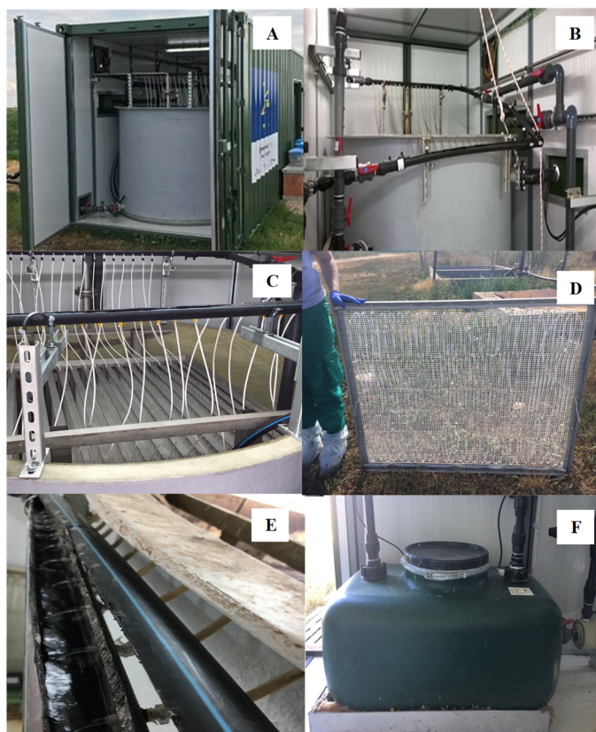
Figure 2. Pictures of the pilot plant. Shipping container, where the mobile pilot plant is located (A), manure tank with 16 membrane parallel panels (B,C), membrane panel (D), open pipeline for trapping solution collection (E), trapping solution tank (F).
