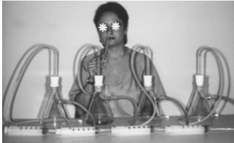
Fig 1. Basic system of subjective olfactometry was used to establish the threshold level. Air was added by syringe to a 500-mL glass vessel containing 50 mL of an odorous solution; the positive pressure then moved the air with odorous molecules toward an exit. The circuit ended in a rubber tube with a final bulb adapted to the patient's nostrils. In this way, when the exit was opened, a known quantity of air with odorous molecules was introduced into the nasal fossa.
