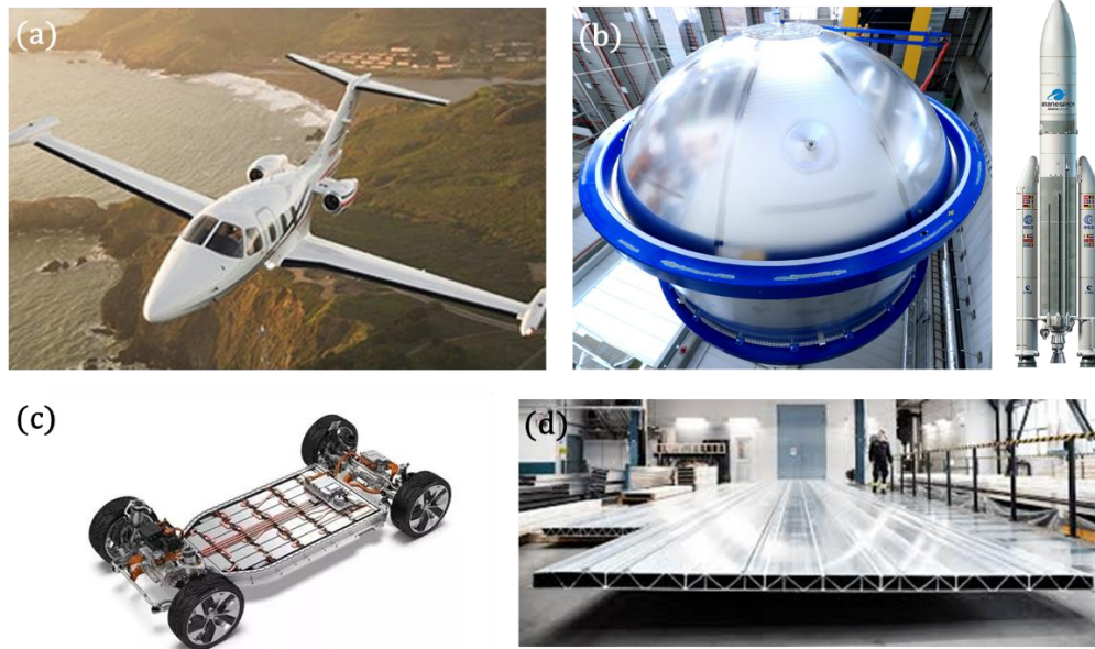
Figure 8 Illustration of FSW applications across various sectors. (a) Aviation: Eclipse 550 aircraft, utilizing FSW for 128 meters of welding, replacing 60% of traditional rivets [117]; (b) Space: Hydrogen tank for the Ariane 6 upper stage [118]; (c) Automotive: Battery trays for electric vehicles [119]; (d) Naval: Floor panels of large high-speed vessels [120].
