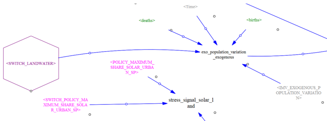
Figure 14 LAND AND WATER SWITCH which isolates Land and Water module from the rest of WILIAM (modularization)
