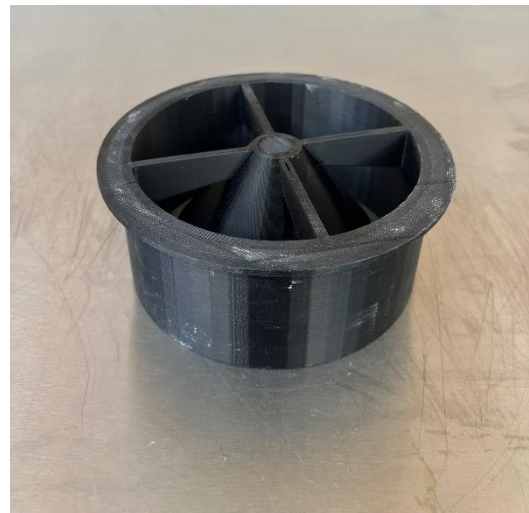
Figure 75: Die made with 3D printing.
