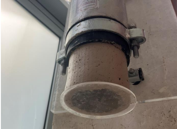
Figure 76: Plastic piece stuck to one side of the extruded piece to facilitate removal.
