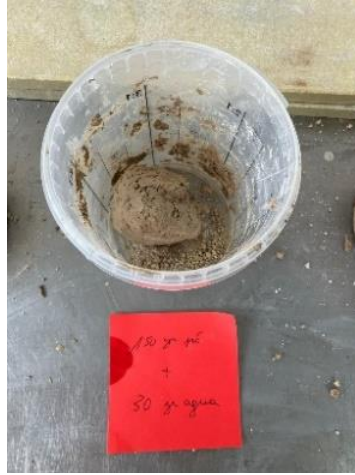
Figure 44: Mixture in vase of 150 grams of powder clay with 30 grams of water.
