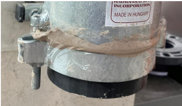
Figure 56: Solution so that the clay does not come out in unwanted places.
