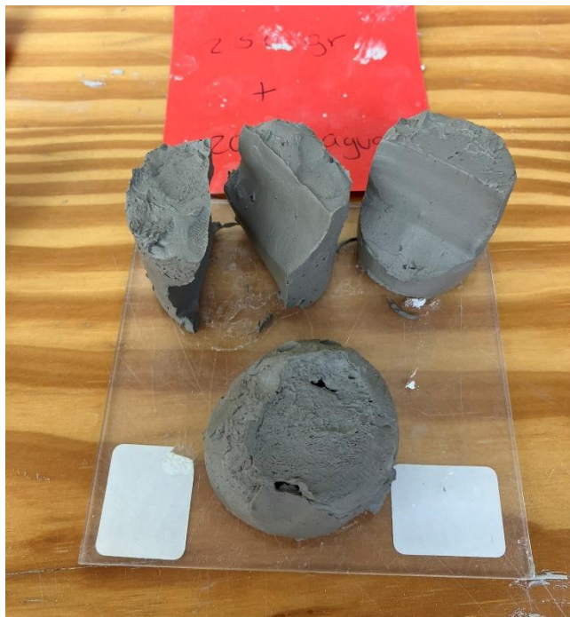
Figure 41: Test with 250 grams of block clay mixed with 20 grams of water.
