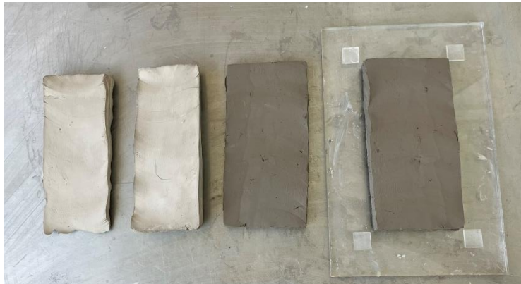
Figure 111: Moulding and wire cut tests.
