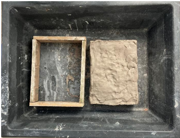
Figure 58: Clay block made with wooden mould.
