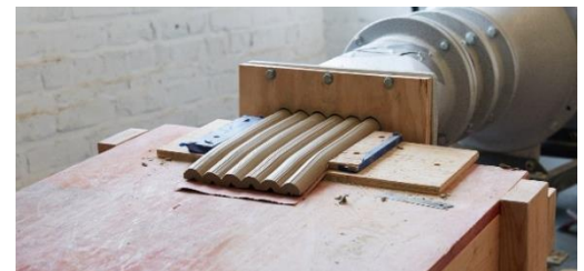
Figure 34: Tiles extrusion process. [27]
