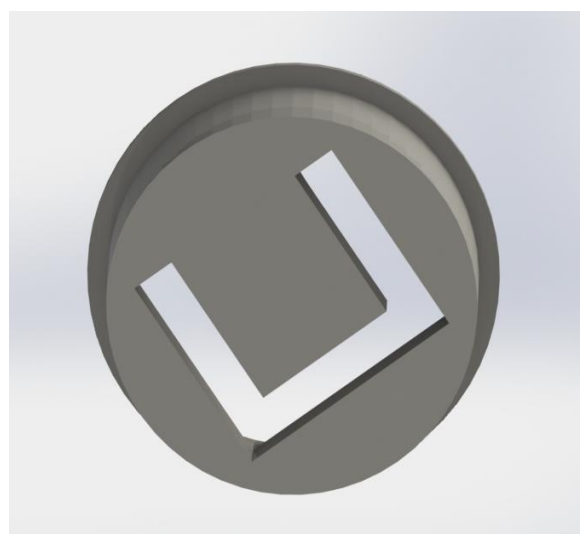
Figure 88: Bottom view of 'U' die.
