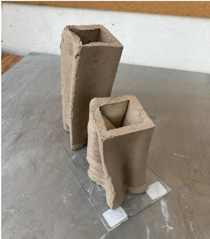
Figure 91: Square die tests.
