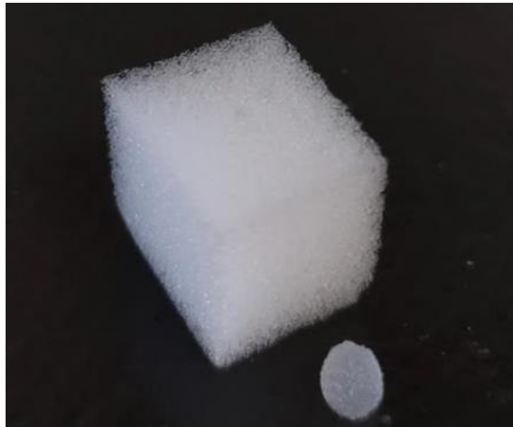
Figure 6. Comparison of original melamine sponge size and after 15 days of trial in MQ water.
