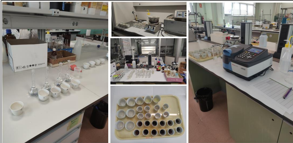
Figure 11. Determination of nitrates by spectrophotometry. From E. Herrero de San Luis©.
