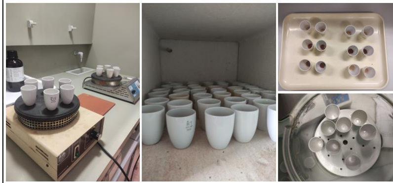
Figure 9. Determination of ash content in wood and bark samples. From E. Herrero de San Luis© and R. C. Martín-Sanz©.
