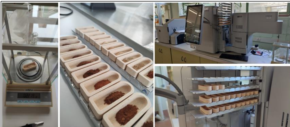
Figure 12. Determination of total C and N by dry combustion using Leco CSN 928 ® elemental analyser. From R. C. Martín Sanz© and E. Herrero de San Luis©.
