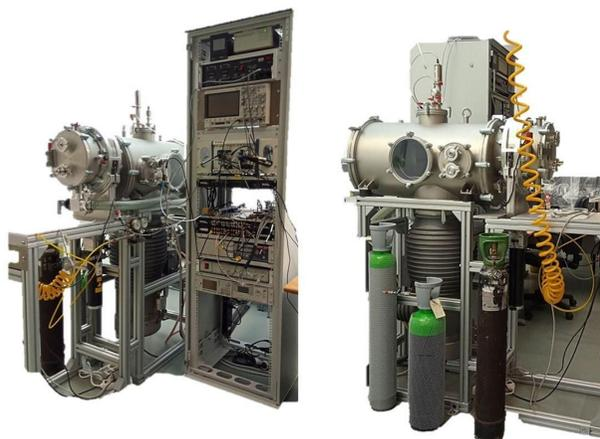
**Figure 1.4** The high-resolution Balle-Flygare Fourier transform microwave spectrometer in our group with the front and side views.
