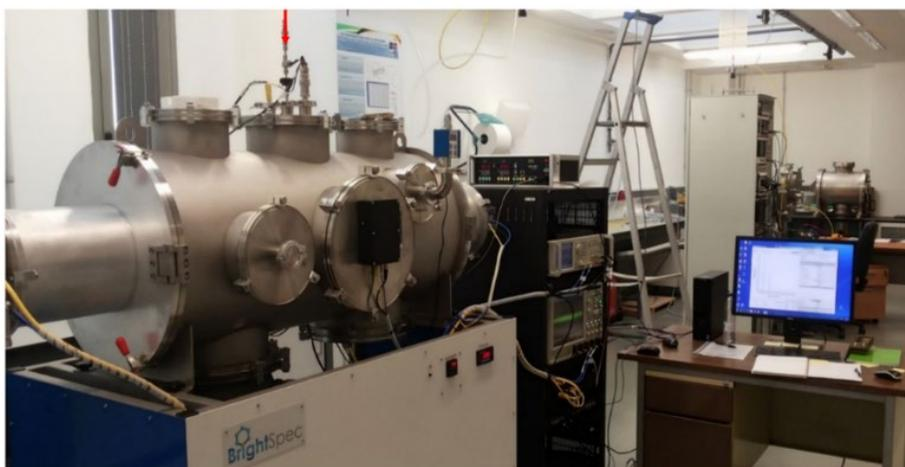
**Figure 1.6** Broadband CP-FTMW spectrometer at Universidad de Valladolid, showing the electronic rack and the expansion chamber. The arrow shows the gas inlet.
