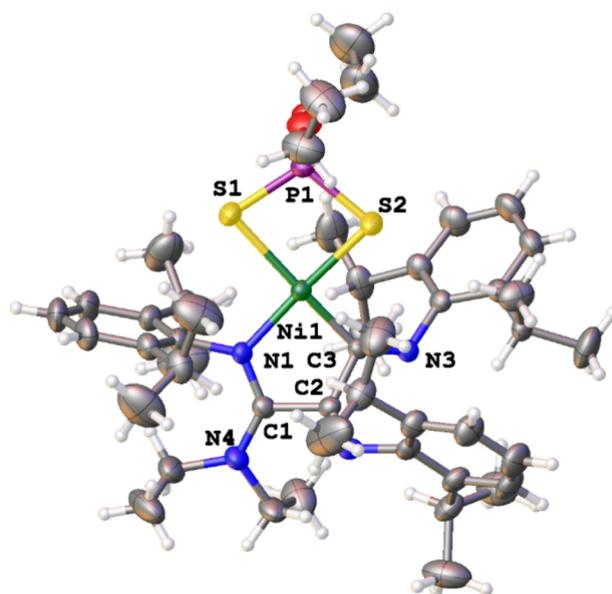
**Figure 1.** X-ray diffraction structure of complex **3a**. Selected bond lengths (Å) and angles (deg): Ni(1)–S(1): 2.3438(9), Ni(1)–S(2): 2.2191(9), Ni(1)–N(1): 1.944(2), Ni(1)–C(3): 1.881(3), S(1)–Ni(1)–S(2): 87.34(3), N(1)–Ni(1)–C(3): 85.41(10).
