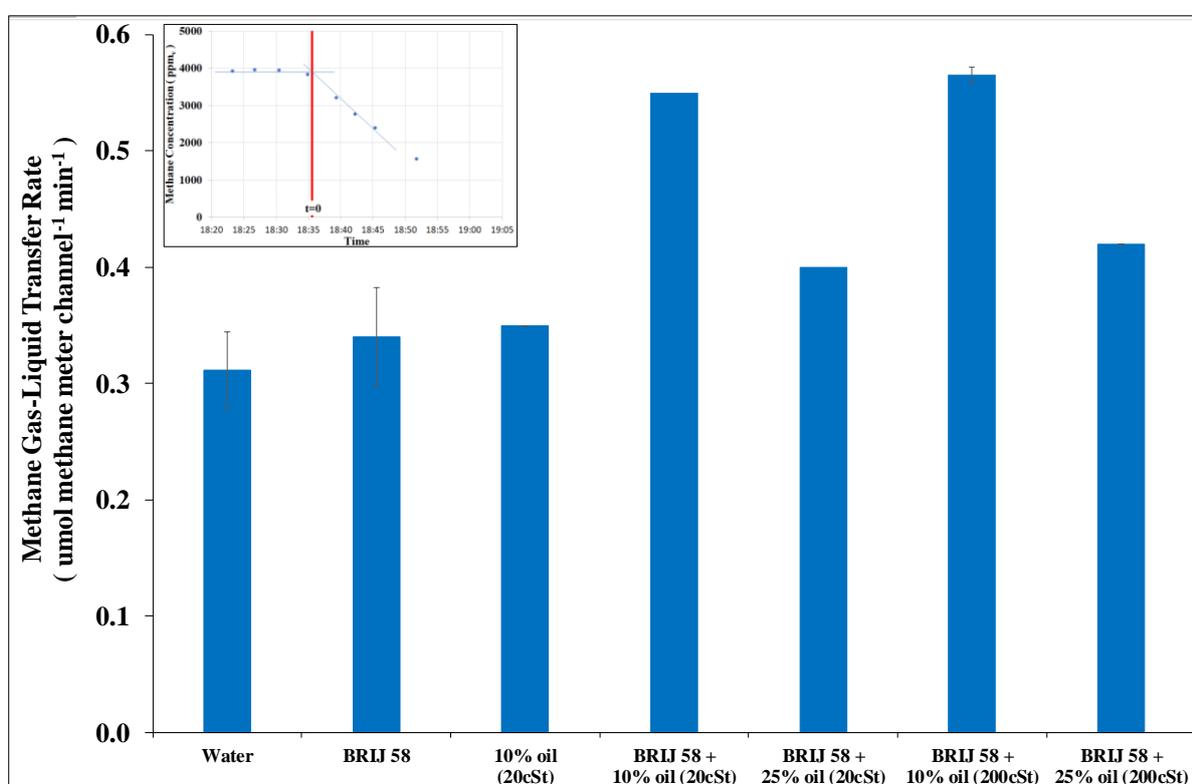
**Figure 8-7** Mass-transfer rate of methane in the single capillary channel with liquids containing different additives. Graphic in the top left corner showing an example of the gaseous methane concentration over time with t=0 the start of the liquid recirculation.
