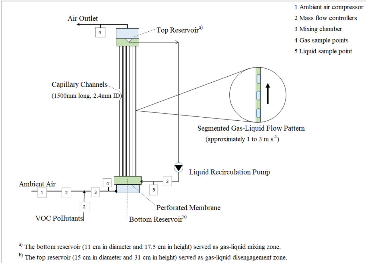
**Figure 5-1** Schematic representation of the experimental set-up of the capillary bioreactor.
