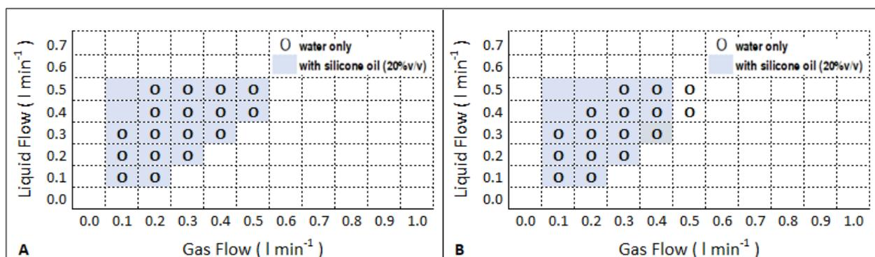
**Figure 6-1** Occurrence of segmented flow in capillary channels with internal diameter of 3.4 mm (A) and 5.0 mm (B) under the different gas flowrate and liquid flowrate conditions using water only and water with silicone oil.
