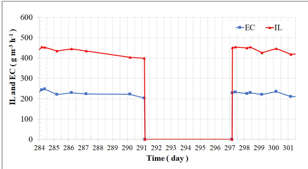
**Figure 9-13** Methane Elimination Capacity (EC) and Inlet load (IL) before and after a six-day methane supply interruption.
