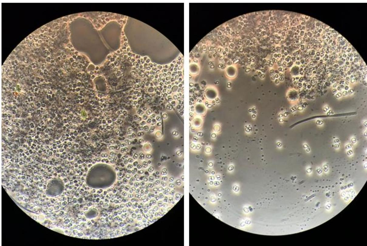
**Figures 9-11** Microscopic (100 x magnification) images of the recirculation liquid of the CBR during Experiment C after the addition of 5% v/v 20 cSt silicone oil (Stage III) about 15 minutes after taking the sample showing small silicone oil conglomerates.
