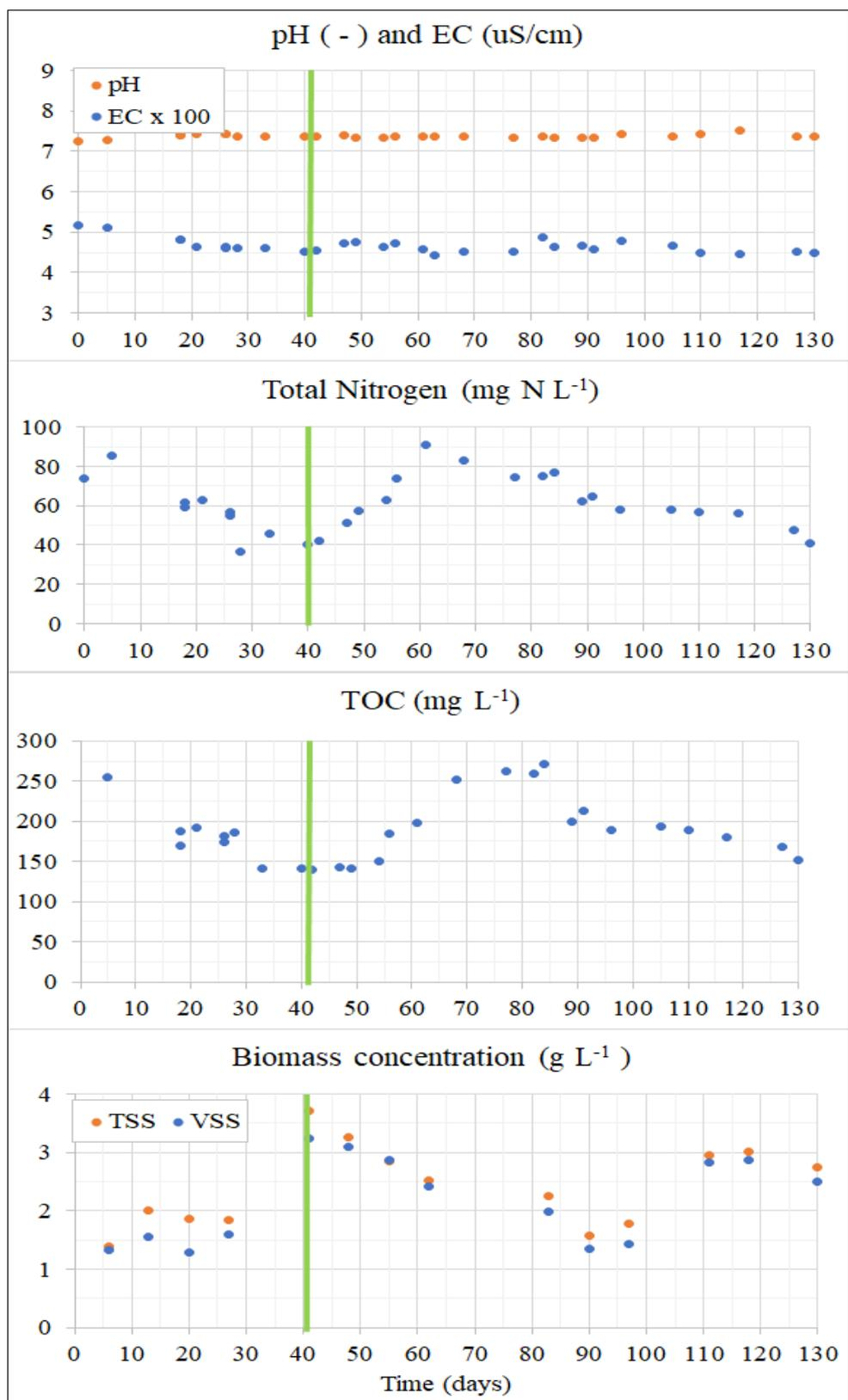
**Figure 9-14** Time course of the results of the aqueous phase analyses during the last 130 days of Experiment C with the green line indicating the addition of nitrogen (40 mg N L<sup>-1</sup> in the form of sodium nitrate).
