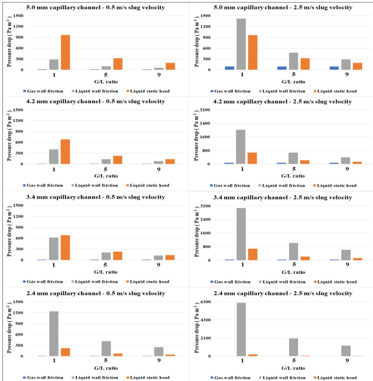
**Figure 9-19:** The pressure drop caused by gas wall friction (blue), liquid wall friction (grey), and liquid static head (red) as a function of the gas-to-liquid ratio for a relatively low slug face velocity (left graphics) and relatively high gas velocities (right graphics) for the following capillary channel different in diameter: 5.0 mm (top), 4.2 mm (upper middle), 3.4 mm (bottom middle), and 2.4 mm (bottom).
