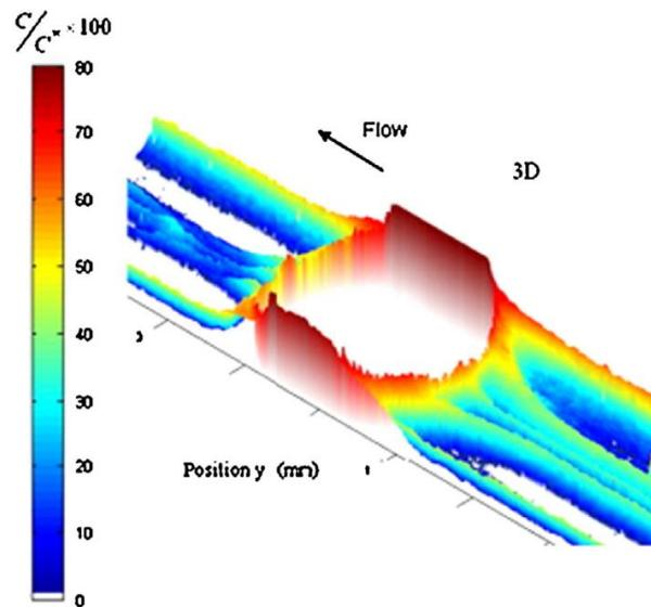
**Figure 11-2** Computational Fluid Dynamics (CFD) visualisation of oxygen concentrations around a phase gas bubble in a capillary channel under segmented (Taylor) flow (courtesy of Dietrich et al., 2013).
