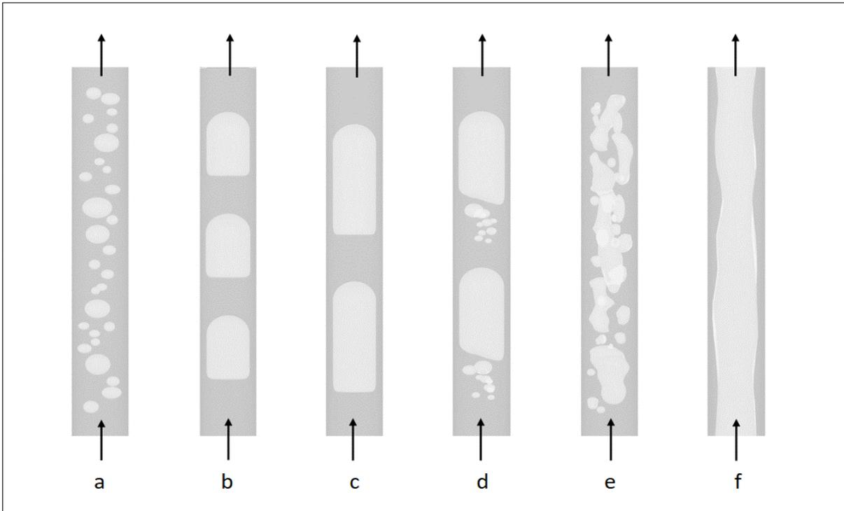
**Figure 5-2** Schematic of possible gas-liquid flow patterns in a capillary channel with (a) bubbly flow, (b, c) segmented flow, (d) transition slug/churn flow, (e) churn flow, (f) falling film flow. (adapted from Kreutzer and co-workers, 2005).
