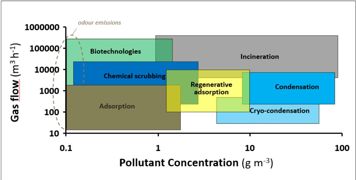
Figure 3-2 Typical application range of gas treatment technologies (adapted from van Groenestijn and Hesselink, 1999).
