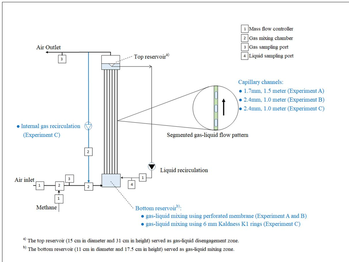
**Figure 9-1** Set-up of the capillary bioreactor to study dilute methane removal.
