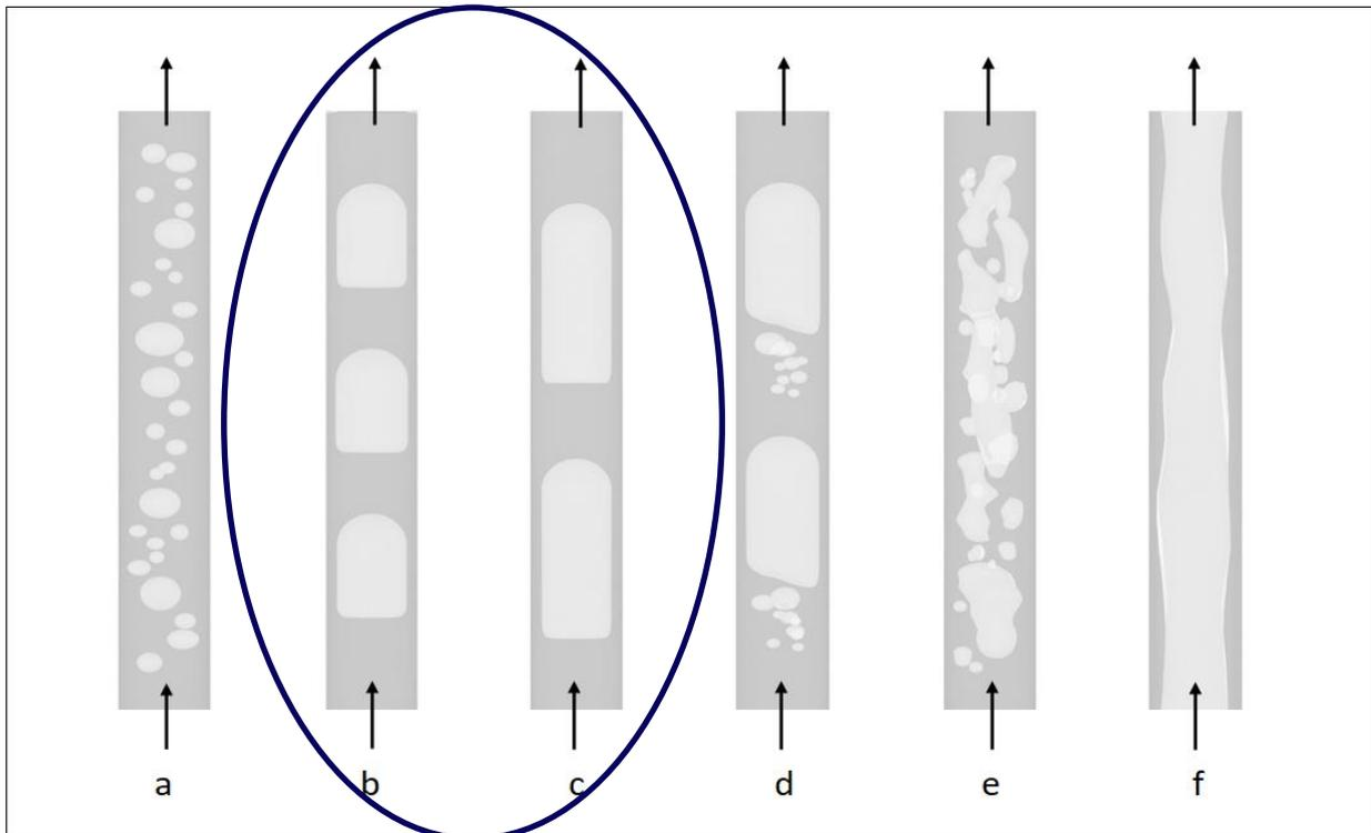
**Figure 4-4** Schematic of possible gas-liquid flow patterns in a capillary channel with (a) bubbly flow, (b, c) segmented flow/slug, (d) transition slug/churn flow, (e) churn flow, (f) falling film flow/annular. (adapted from Kreutzer and co-workers, 2005b).
