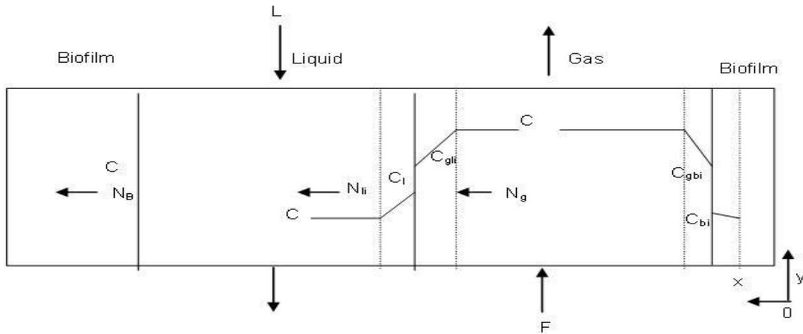
**Figure 4-1** Illustration of mass transfer typical for biological gas treatment processes (Kraakman et al., 2011).
