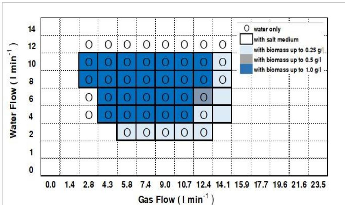
Figure 5-4 Occurrence of segmented flow in the capillary reactor in all the twenty-five channels under the different gas flowrate and liquid flowrate conditions using water only, salt medium and biomass additions to the mineral salt medium.
