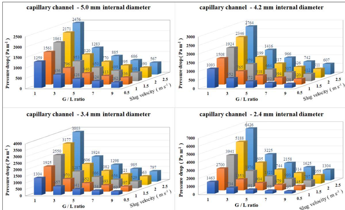
**Figure 9-18:** The pressure drop as a function of the gas-to-liquid ratio and the slug face velocity for the following capillary channel different in diameter: 5.0 mm (top left), 4.2 mm (top right), 3.4 mm (bottom left), and 2.4 mm (bottom right).
