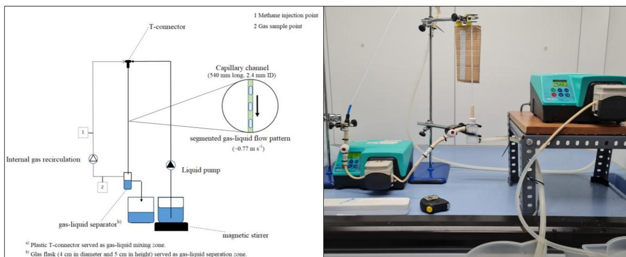
**Figure 8-3** Schematic representation of the experimental set-up (left) and the actual set-up of the single capillary channel mass transfer measurements.
