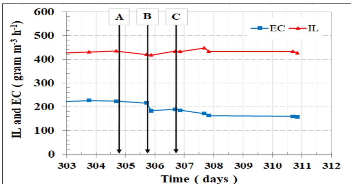
**Figure 9-15.** Effect of additional BRIJ 58 on the methane Elimination Capacity (EC) at the relatively constant Inlet Load (IL) during the final phase of the experiment with (A) the additional 80 mg BRIJ 58 L<sup>-1</sup>, (B) the additional 160 mg BRIJ 58 L<sup>-1</sup>, and (C) the additional 320 mg BRIJ 58 L<sup>-1</sup>.
