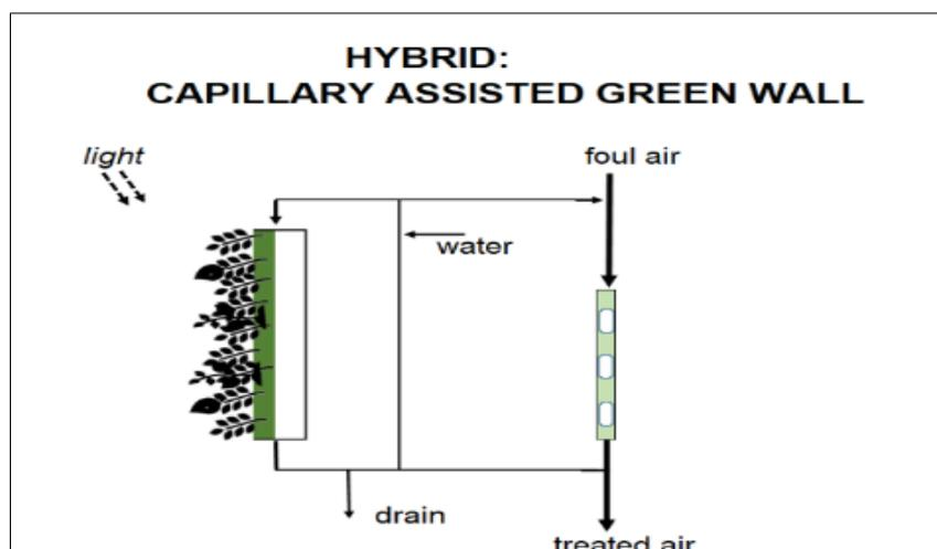
**Figure 11-3** Sketch of the concept of a capillary reactor combined with a green wall.
