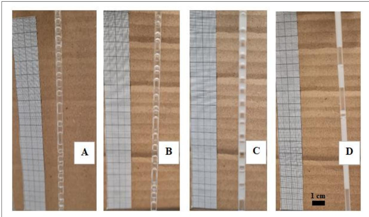
**Figure 8-8** Photos of the segmented flow patrons in the single capillary channel during the abiotic mass-transfer rate experiment of water only (A), water + BRIJ 58 (B), water + BRIJ 58 + 10 % v/v silicone oil (C), and water + BRIJ 58 + 25 % v/v silicone oil (D).
