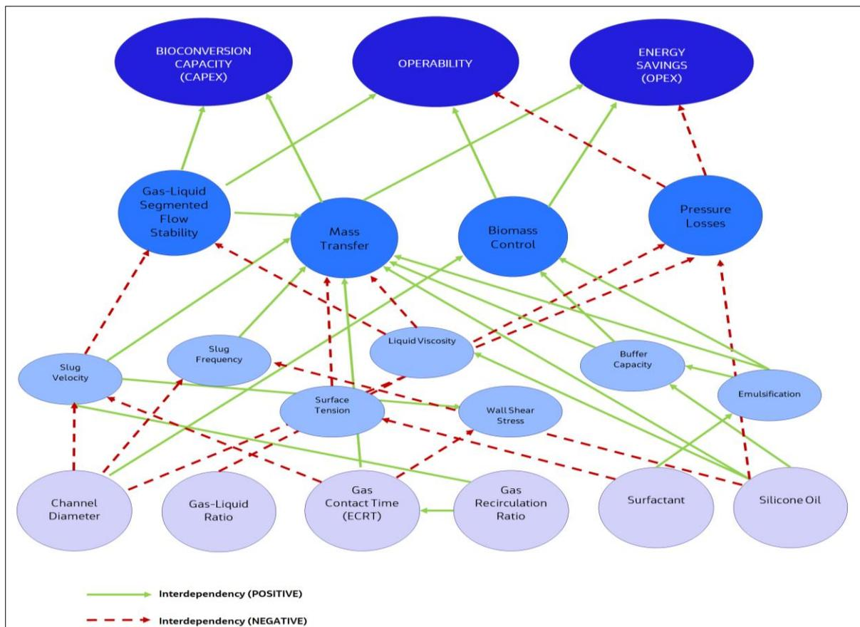
**Figure 11-1** Schematic presentation of the interdependent relations between capillary bioreactor designs inputs (bottom) and relevant economic functionality outputs (top).
