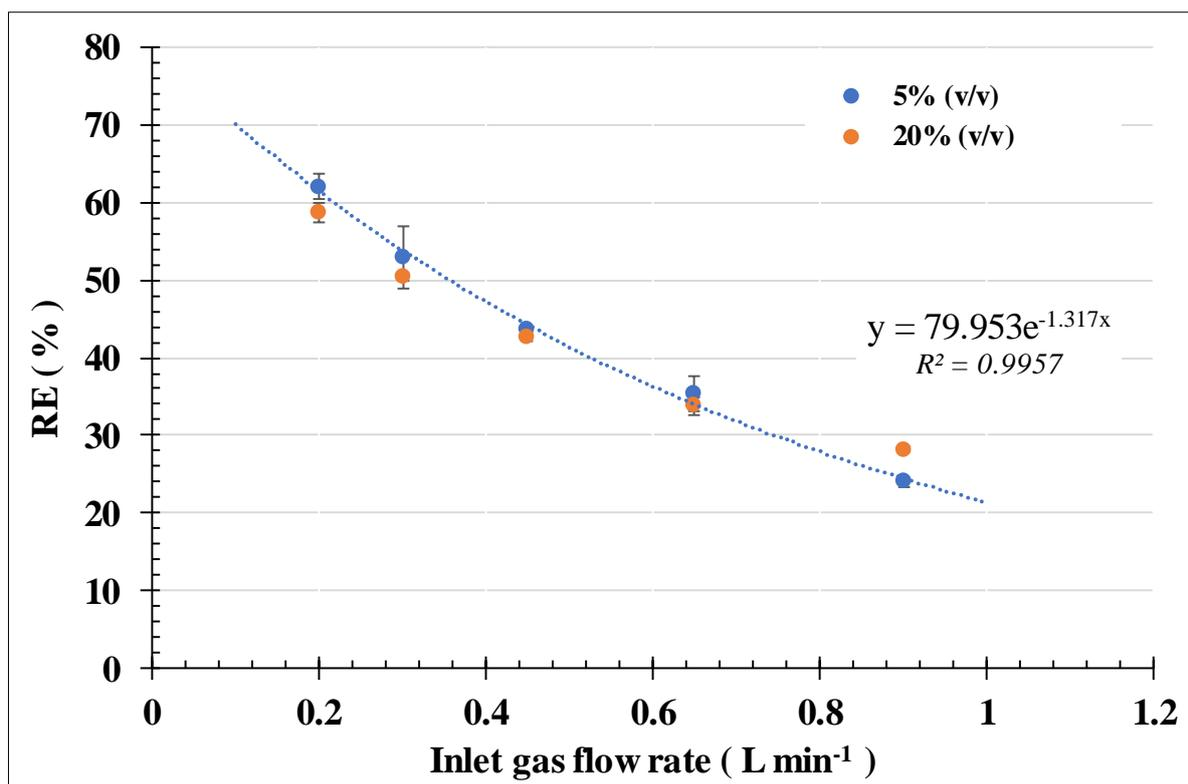
**Figure 9-5** Methane removal efficiency in the capillary bioreactor operated at a constant inlet methane loading rate and constant channel gas-liquid slug velocity while only the inlet gas flow rate was increased resulting in reduced internal gas recirculation rates and reduced overall gas contact time, and reduced inlet methane concentration during Stage IV (5% v/v oil) and Stage V (20% v/v oil).
