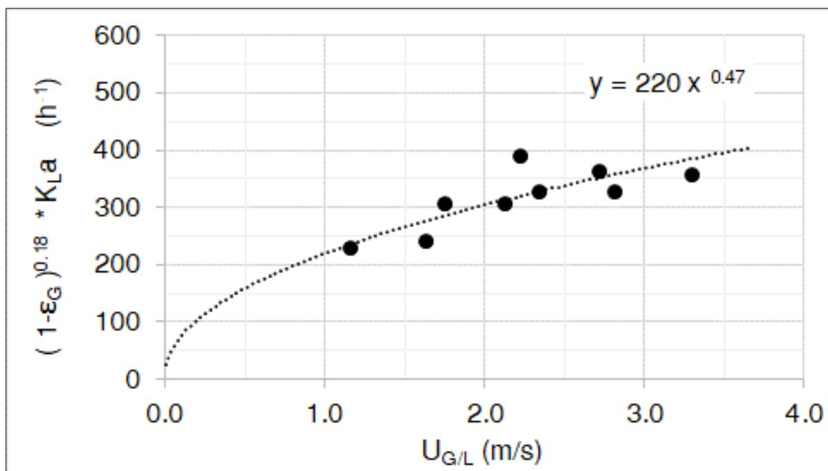
**Figure 5-5** Correlation of the mass transfer data to the gas bubble-liquid slug superficial velocity ( $U_{G/L}$ ) and the average gas volume fraction ( $\epsilon_G$ ) of the gas bubble-liquid slug.
