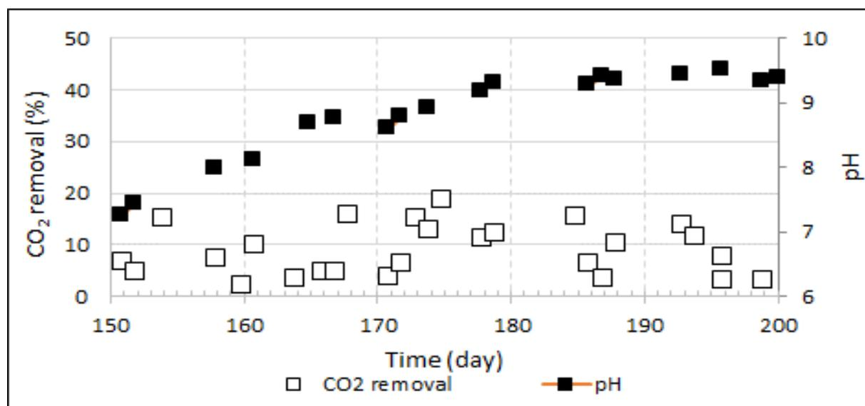
**Figure 7-1** Time course of the removal efficiencies (□) of CO<sub>2</sub> and the pH (■) in the capillary photobioreactor during Phase II (day 150 – 200).
