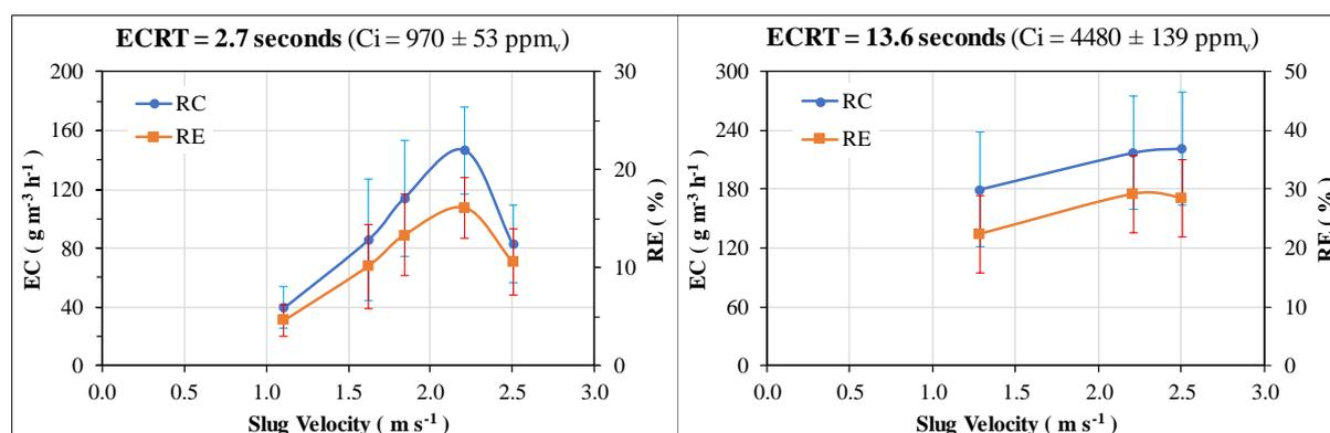
**Figures 9-2.** Methane removal efficiency and methane elimination capacity at 2.7 s of gas contact time (left) and 13.6 seconds gas contact time (right) during the initial 130 days of Experiment C.
