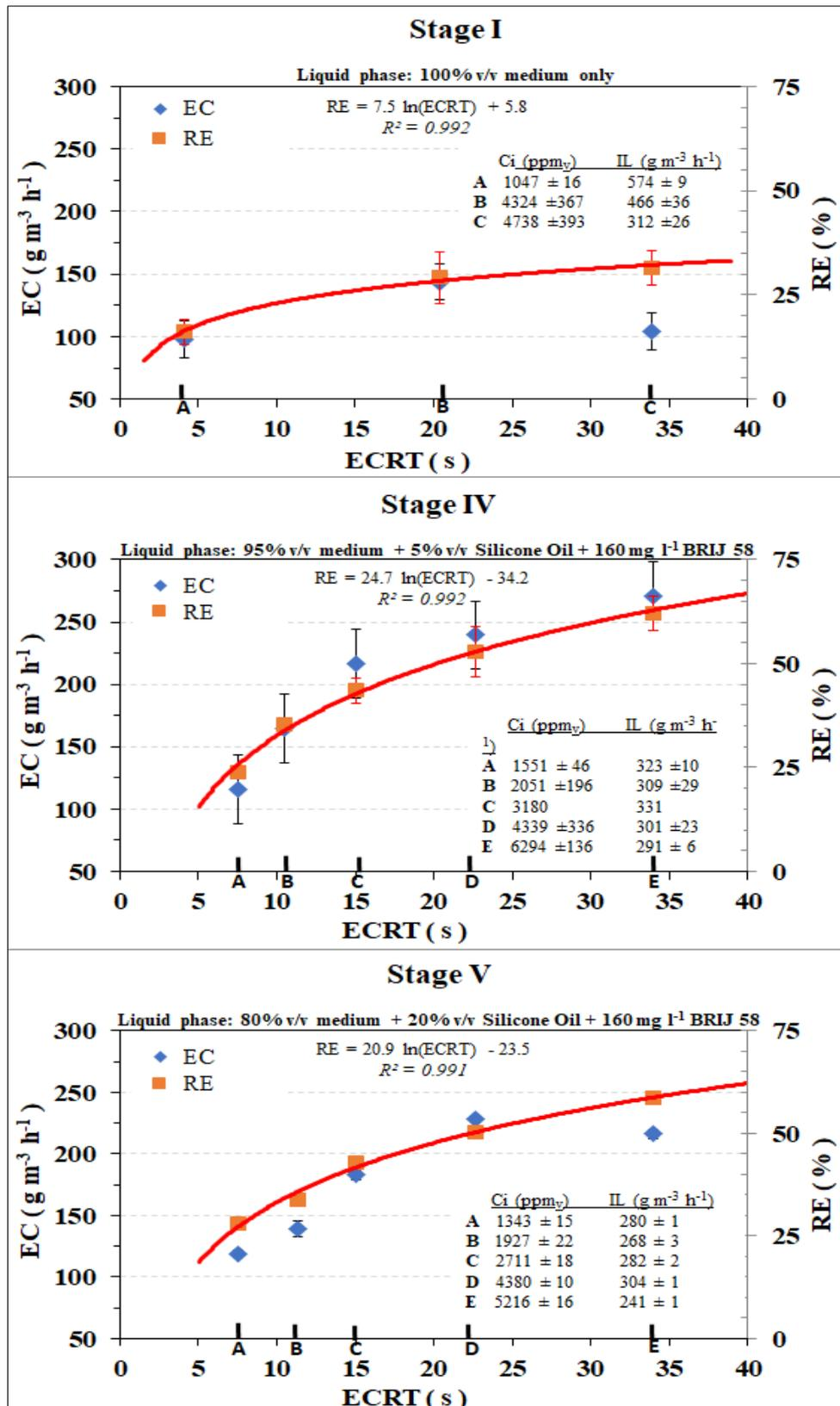
Figure 9-6 Methane removal efficiency (RE) and methane elimination capacity (EC) in the capillary bioreactor during Stage I (upper), Stage IV (middle), and Stage V (lower), and operated under different internal gas recirculation rates resulting in different overall gas contact times and different inlet concentrations.
