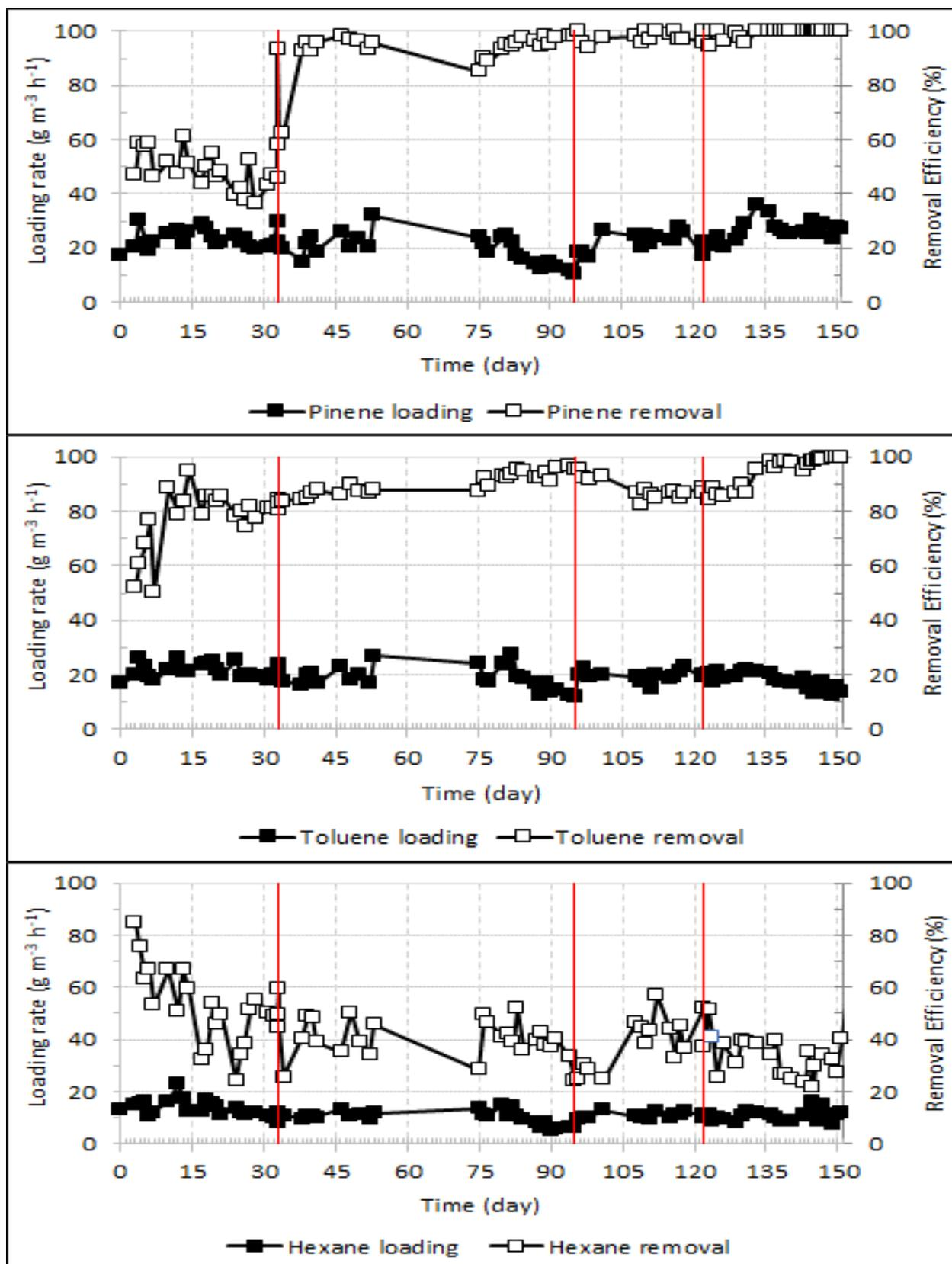
**Figure 6-2** Time course of the loadings rate (■) and removal efficiencies (□) of  $\alpha$ -pinene (upper), toluene (middle) and hexane (lower) in the capillary bioreactor, with the vertical lines the days at which key operating changes were introduced: addition of 5% (v/v) silicone oil (day 33), increased to 10% (v/v) silicone oil (day 95), and increase gas-to-liquid ratio (day 122).
