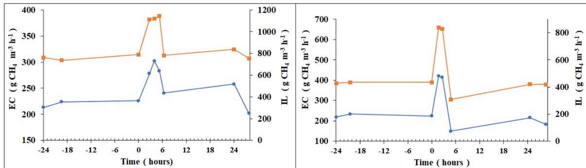
**Figures 9-3** Methane (●) elimination capacity (EC) and the methane (■) inlet load (IL) in the capillary bioreactor during the mass transfer limitation test before (Stage I, Figure 9-2a, left) and after (Stage V, Figure 9-2b, right) the supplementation of additives to the liquid phase.
