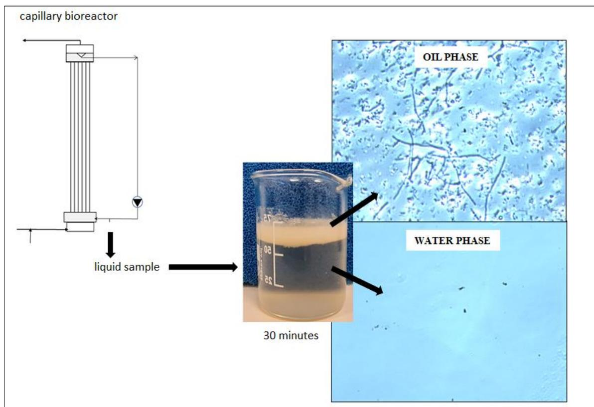
**Figure 6-3** Photos of the microbial appearance in the recirculation liquid of the capillary bioreactor at the end of Phase I after separating the two-liquid phases.
