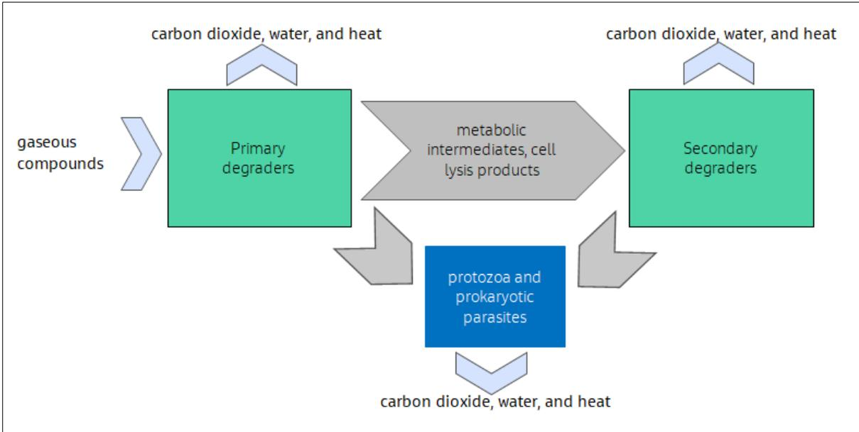
Figure 3-1 Typical bioconversion process in an aerobic biological gaseous treatment system.
