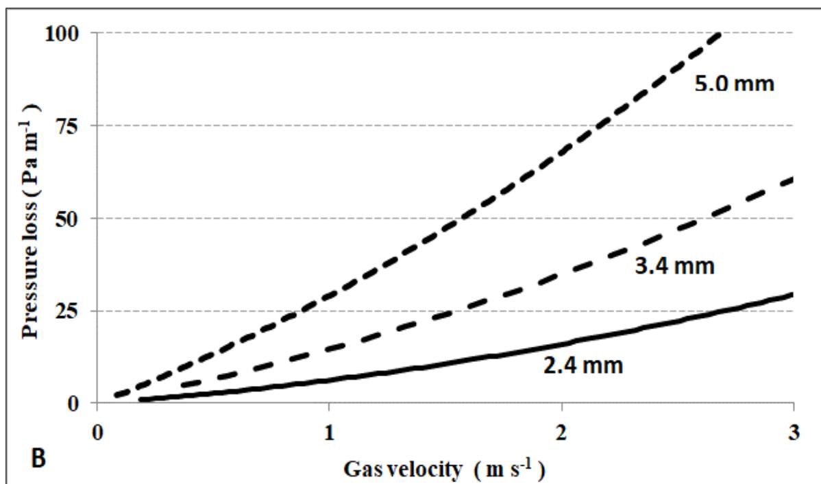
**Figures 5-3** The pressure loss per meter of glass channel of ambient air flowing through glass channels with an internal diameter of 2.4, 3.4 and 5.0 mm as a function of the superficial gas velocity.
