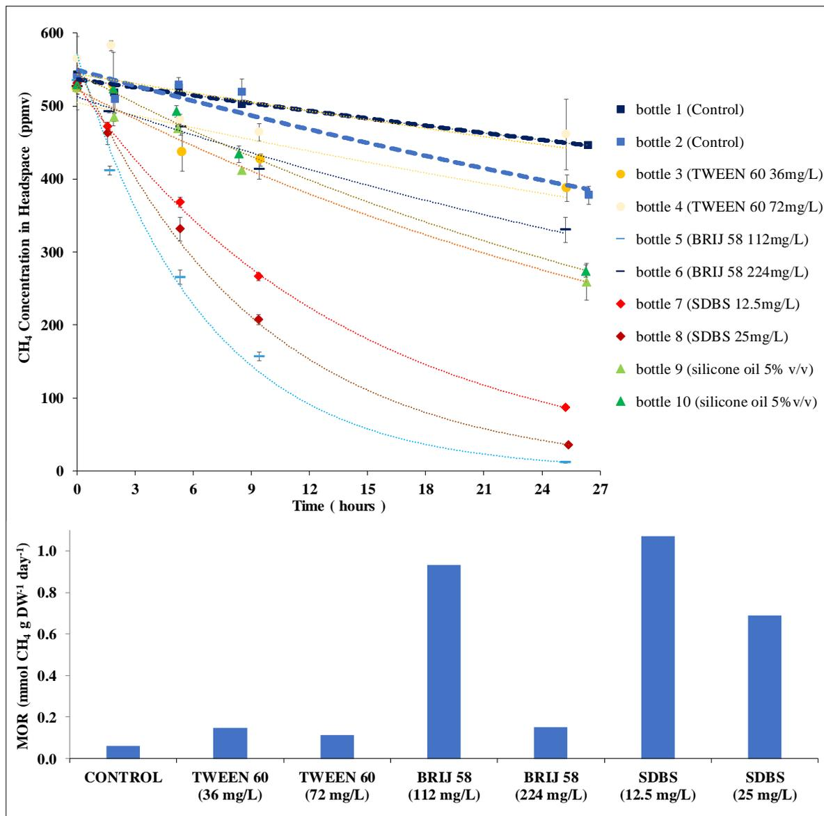
**Figure 8-4** Time course of the reduction of the methane concentration in the headspace of the bottles (upper graphic) and maximum specific methane oxidation rate (MOR) (lower graphic) after 10 weeks containing methane oxidizing microorganisms and different liquid phase additives.
