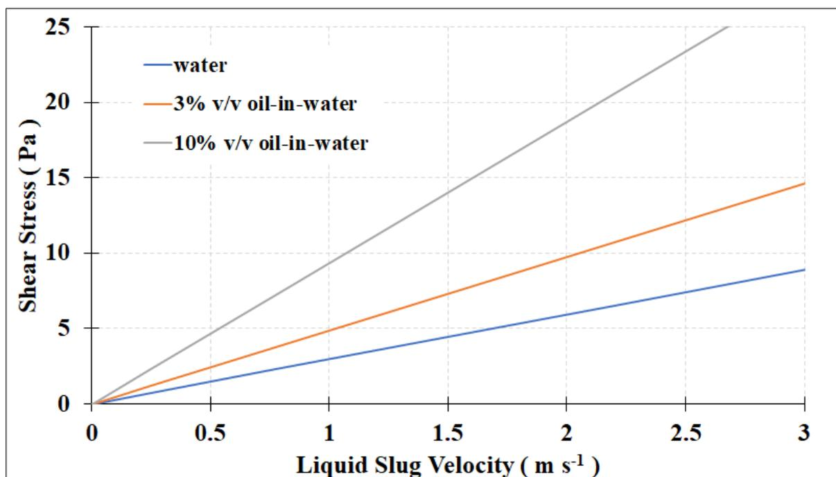
**Figure 9-16** The wall shear stress in the liquid slug in the 2.4 mm capillary channel as a function of liquid superficial velocity for water (viscosity 0.89 mPa s) and two oil-in-water emulsions (oil viscosity 20 cSt = 20 mPa s).
