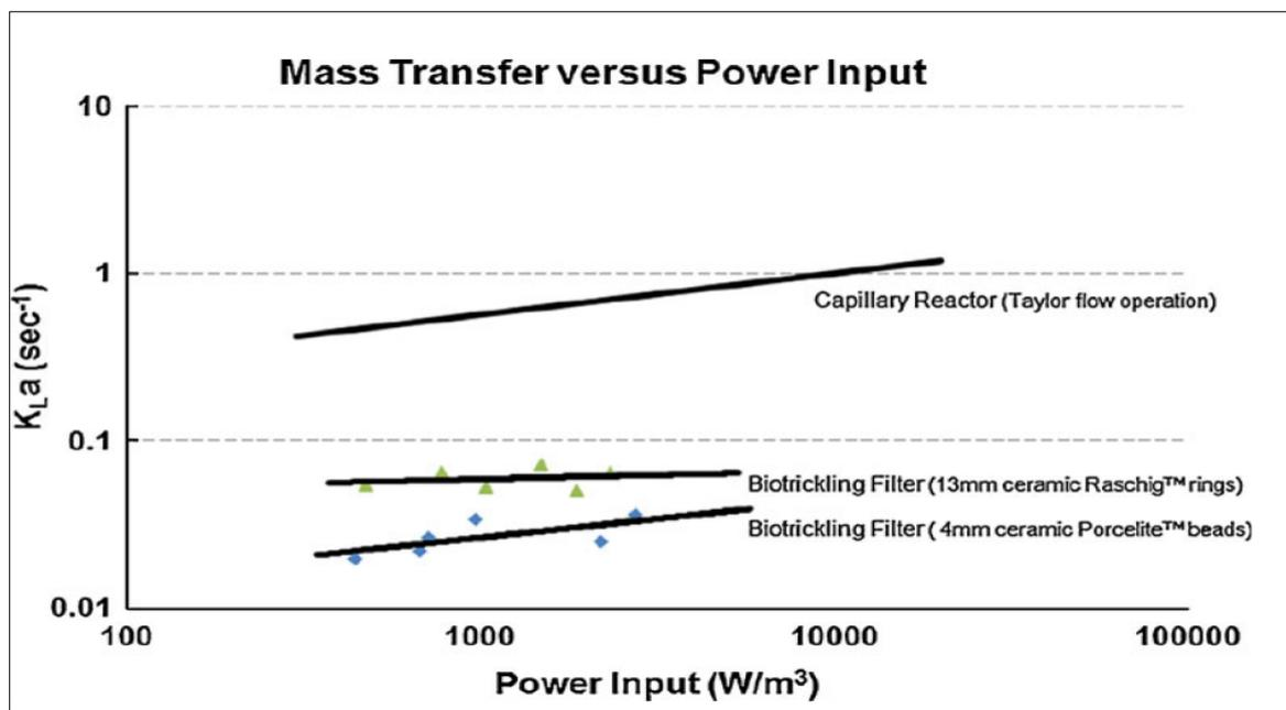
**Figure 4-6** Mass transfer and power consumption in capillary reactor operated under segmented flow regime compared to biotrickling filters (Kraakman et al., 2011).
