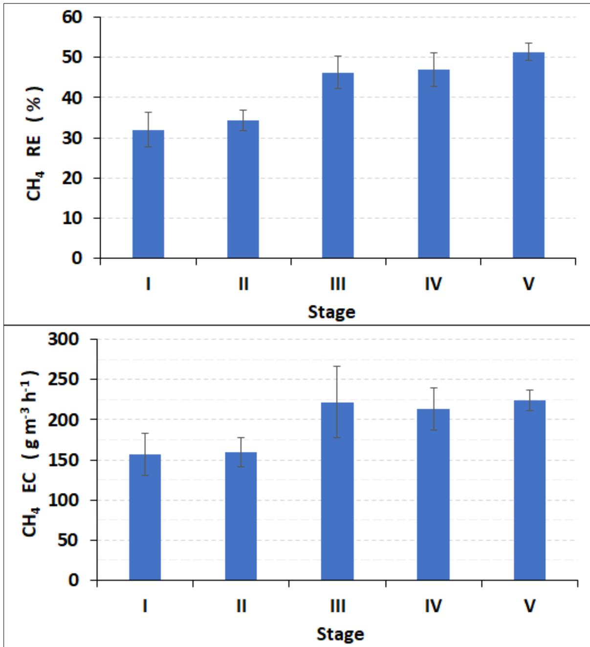
Figure 9-4. Methane removal efficiency (upper) and methane elimination capacity (lower) in the capillary bioreactor during the different experimental stages of quantifying the influence surfactant and silicone oil addition.
