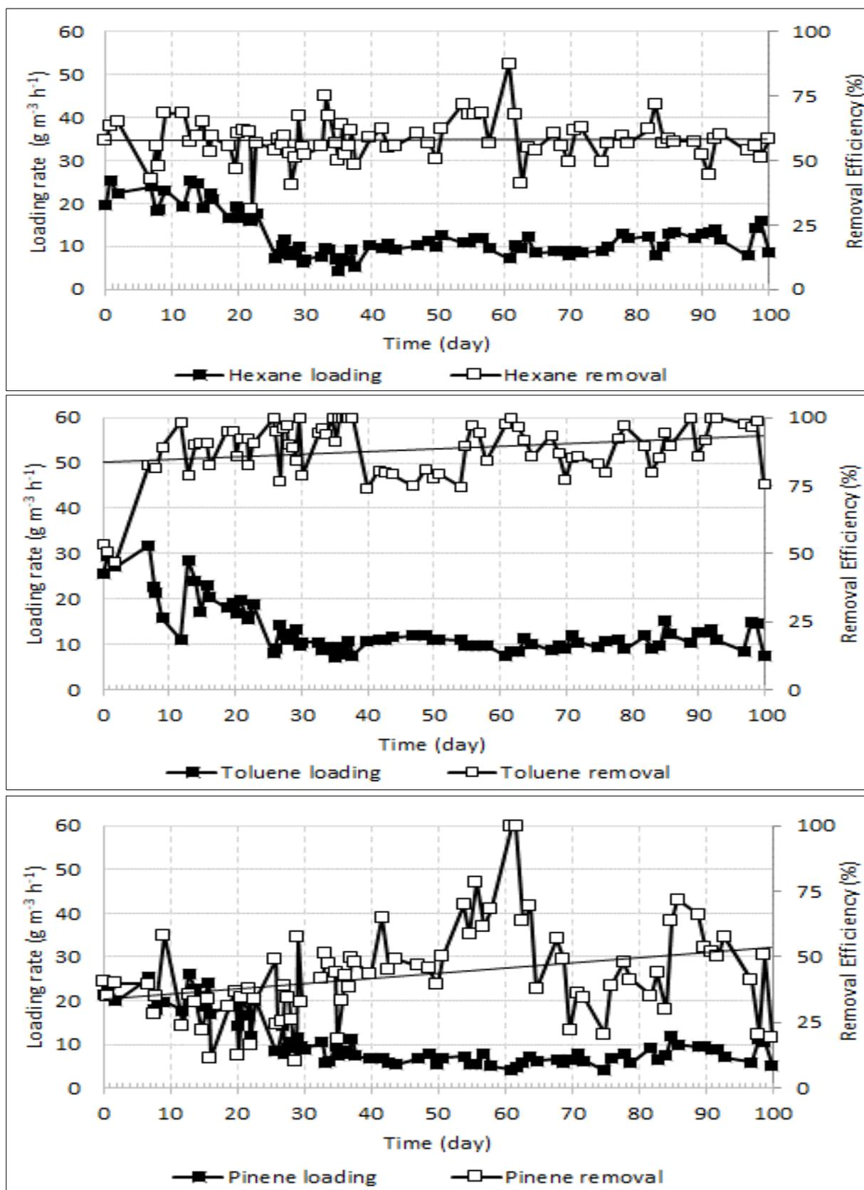
**Figure 5-6** Time course of the loadings rate (■) and removal efficiencies (□) of hexane (upper), toluene (middle) and  $\alpha$ -pinene (lower) in the capillary bioreactor during Phase 1 (day 0 – 25) and Phase 2 (day 25 – 100). The straight line shows the overarching trend of the removal efficiency during the 100-day testing period.
