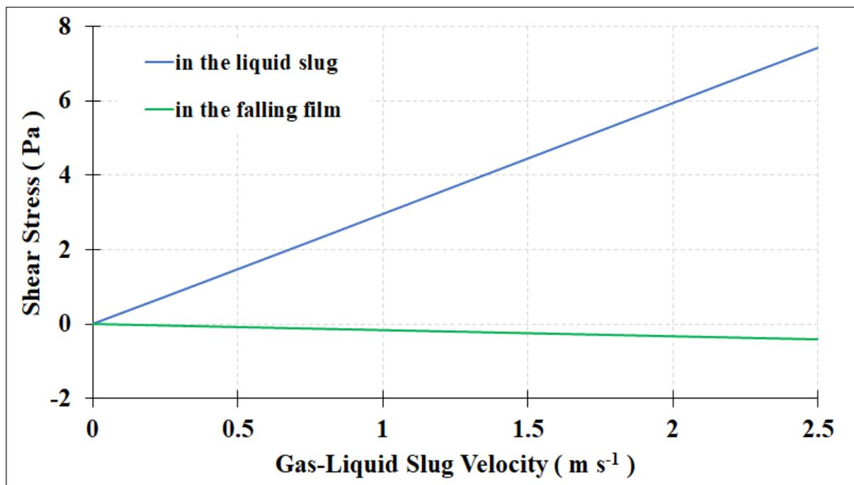
**Figure 9-17** The wall shear stress in the liquid slug and in the falling film along gas bubble in the 2.4 mm capillary channel under segmented flow conditions as a function of gas-liquid superficial velocity for water.
