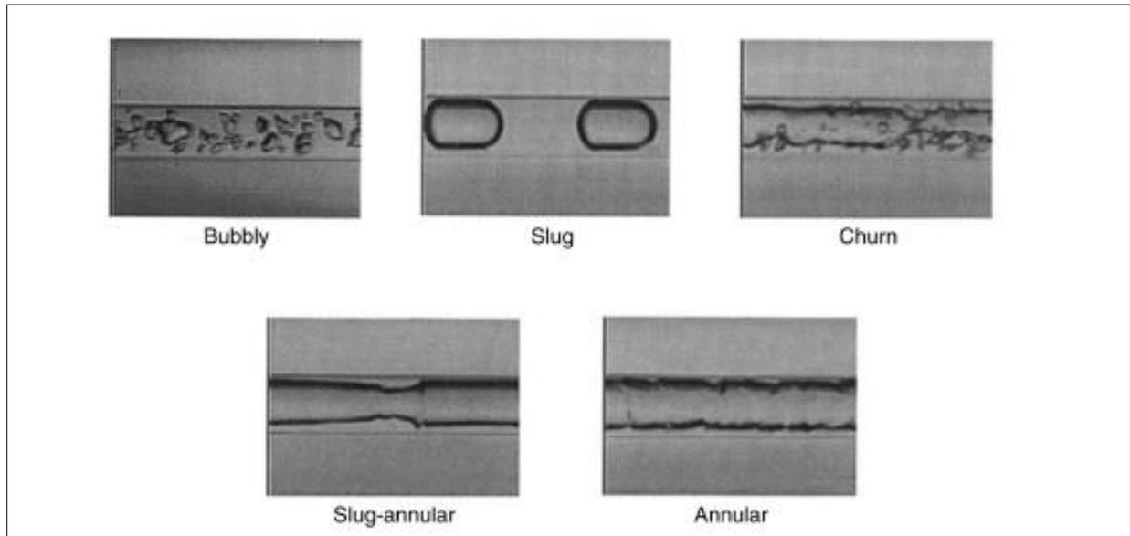
**Figure 4-5** Examples of gas-liquid flow patterns in a capillary channel of 1 mm diameter (Triplett et al. 1999).
