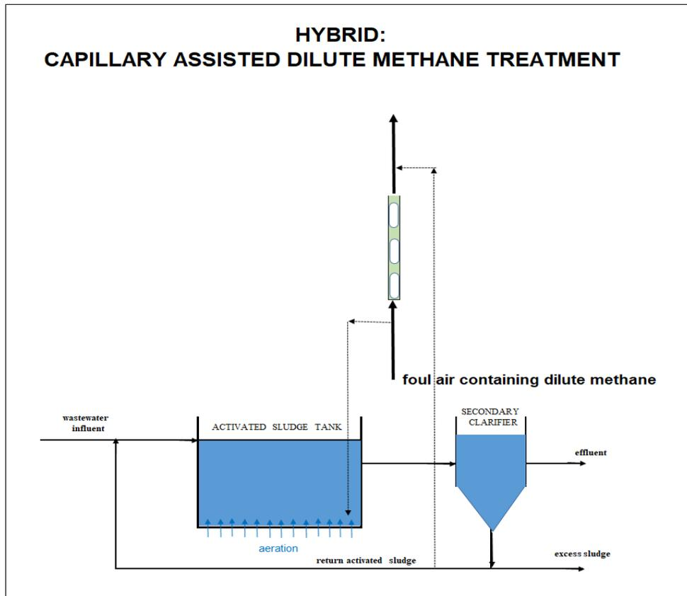
Figure 11-5 Sketch of the concept of a capillary reactor combined with an existing activated sludge tank.
