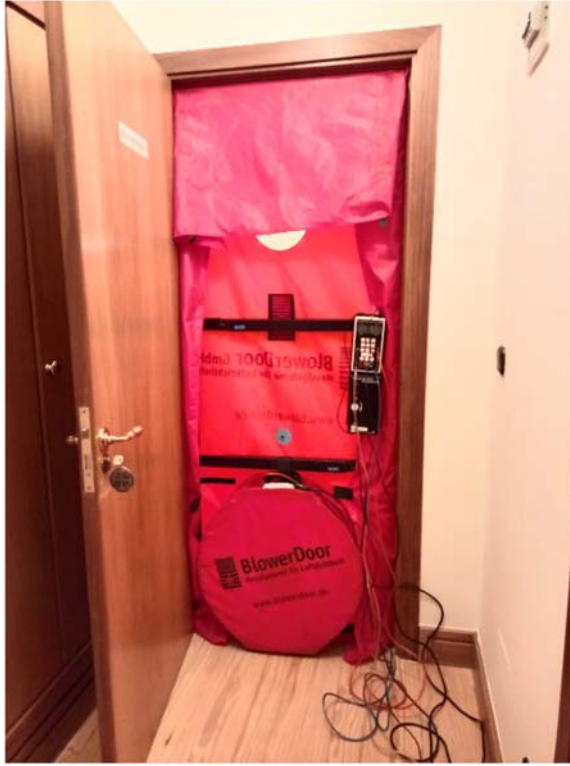
Figure 3.10 Airtightness test layout. Blower door system.
