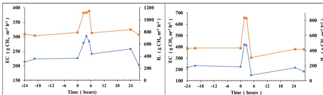
Fig. 6. Methane (●) elimination capacity (EC) and the methane (■) inlet load (IL) in the capillary bioreactor during the mass transfer limitation test before (Stage I, Fig. 6a, left) and after (Stage V, Fig. 6b, right) the supplementation of additives to the liquid phase.
