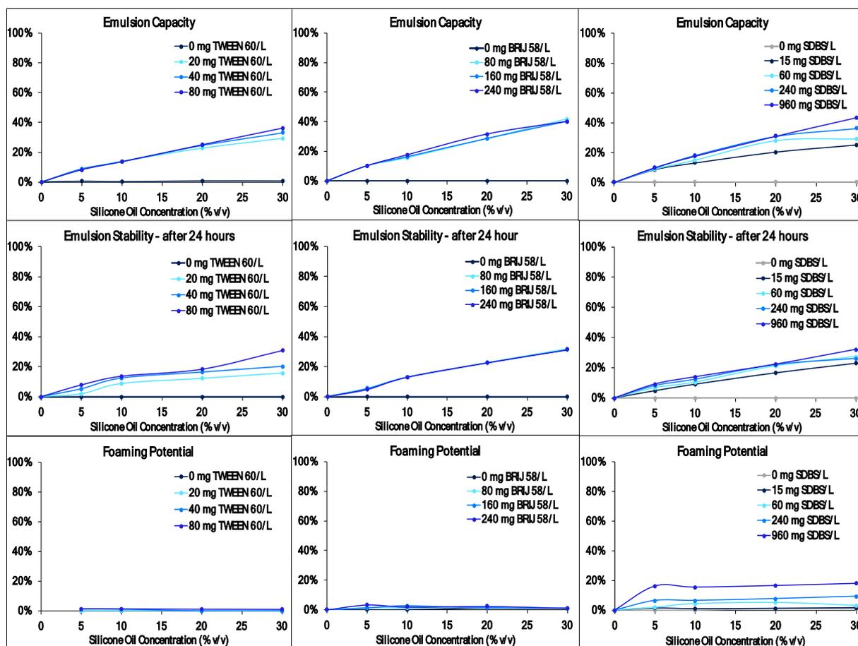
Fig. 4. The Emulsion Capacity (top), Emulsion Stability (middle), and Foaming Potential (bottom) of TWEEN 60 (left), BRIJ 58 (middle), and SDBS (right) at increasing silicone oil percentages.
