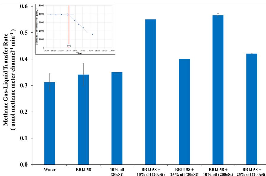
Fig. 5. Mass-transfer rate of methane in the single capillary channel with liquids containing different additives. Graphic in the top left corner showing an example of the gaseous methane concentration over time with  $t = 0$  the start of the liquid recirculation.
