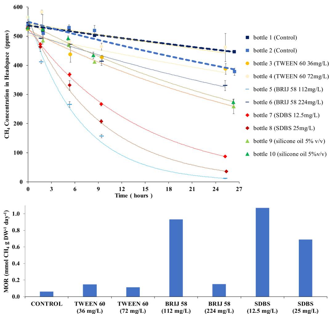
Fig. 2. Time course of the reduction of the methane concentration in the headspace of the bottles (upper graphic) and maximum specific methane oxidation rate (MOR) (lower graphic) after 10 weeks containing methane oxidizing microorganisms and different liquid phase additives. The controls (duplicate) in the upper graphic are shown in bold. The dotted lines were determined through exponential regression ( $R^2 > 0.9$  in all cases).
