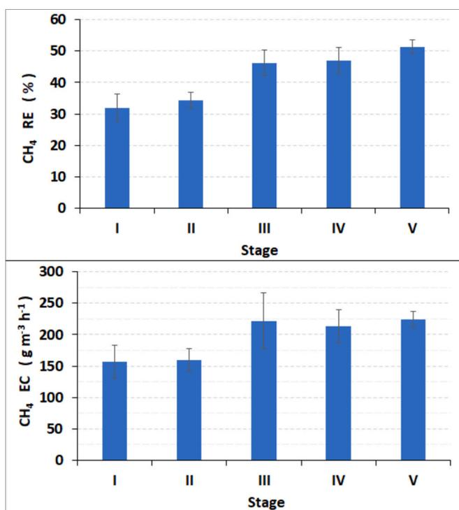
Fig. 7. Methane removal efficiency (upper) and methane elimination capacity (lower) in the capillary bioreactor during the different experimental stages.
