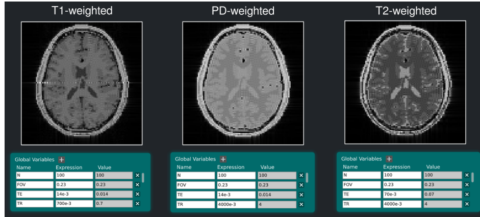
Figure 4.34: MRI simulation results based on the SE sequence created in the GUI. The bottom panels display the global variables of the sequence, with a particular focus on TE and TR, which were adjusted to obtain T_1 , PD, and T_2 -weighted images, respectively.
