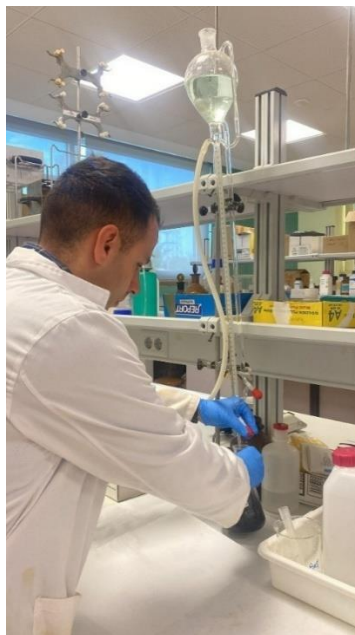
Figure 24. Assessment of dichromate in the determination of organic carbon using the Walkley-Black method
