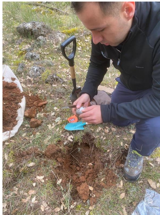
Figure 18. Preparation of soil core samples by trimming excess material prior to sealing.
