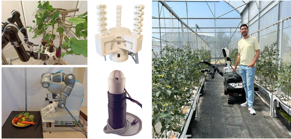
Fig. 5.1.: Proposed soft grippers designs and their implementation in dual-arm robotic systems.
