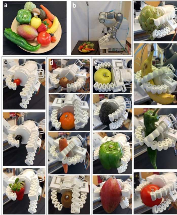
Fig. 4.14.: Soft gripper validation. (a) Fruits and vegetables grasped; their properties are listed in Table 4.3. (b) Experimental setup. (c) Fruits and vegetables grasped using one finger and the palm. (d) Fruits and vegetables grasped using two finger and the palm. (e) Fruits and vegetables grasped with a full grip.
