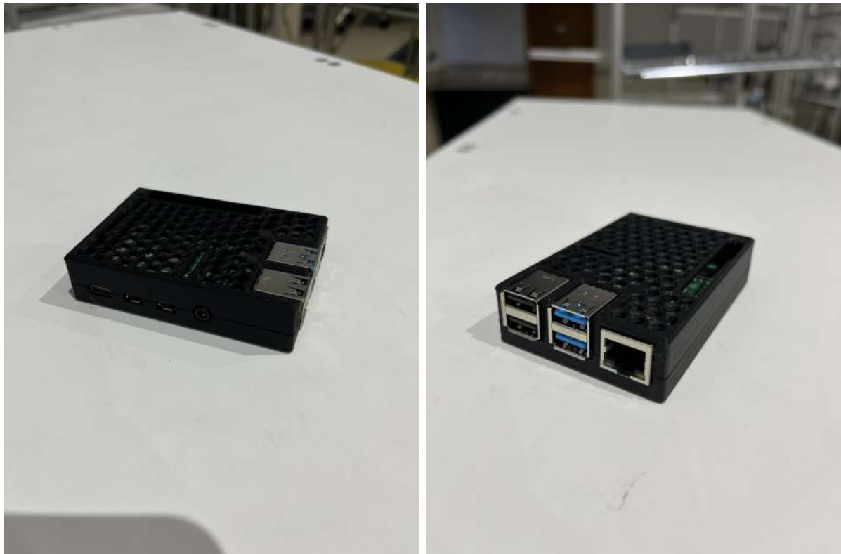
Figure 4.17: Different views of the warehouse's Raspberry Pi in its 3D printed case
