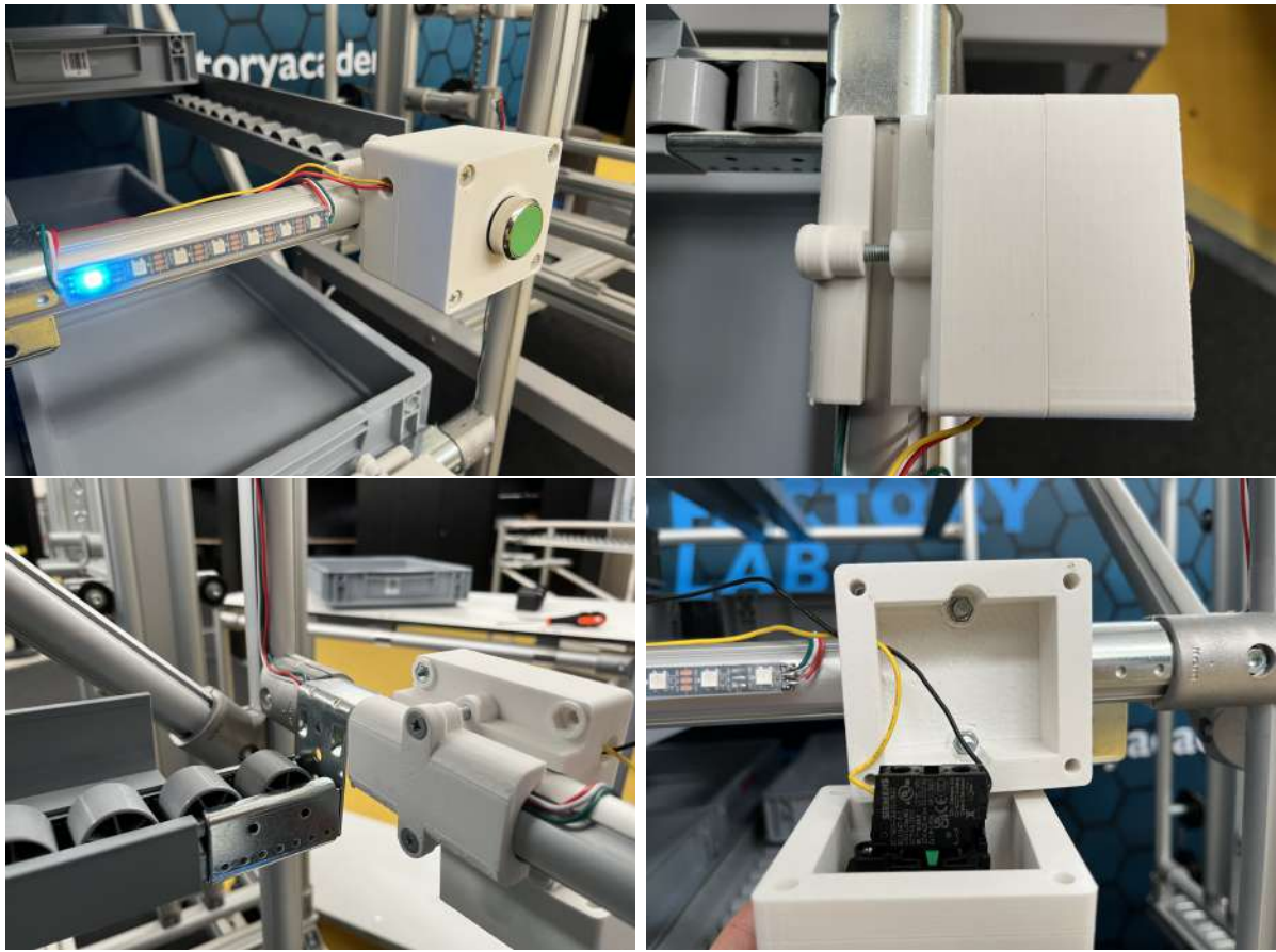
Figure 4.18: Different views of the installation of the button's boxes and the LED strips on the storage rack
