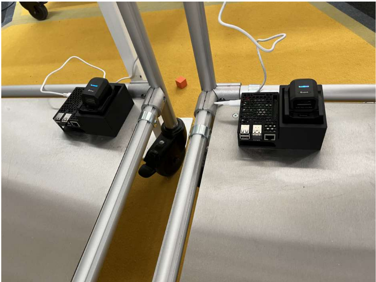
Figure 4.21: System for barcode scanning installed on the bottom shelf of each of the two workstations.
