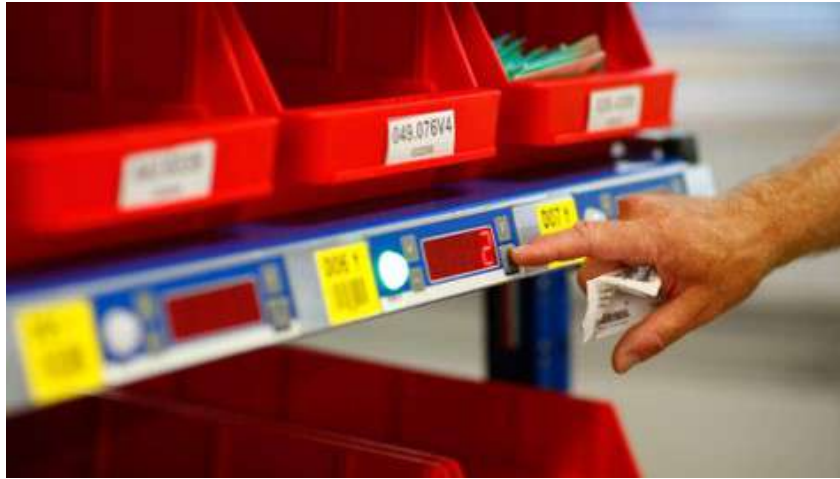
Figure 3.7: Pick to light system in a warehouse.
