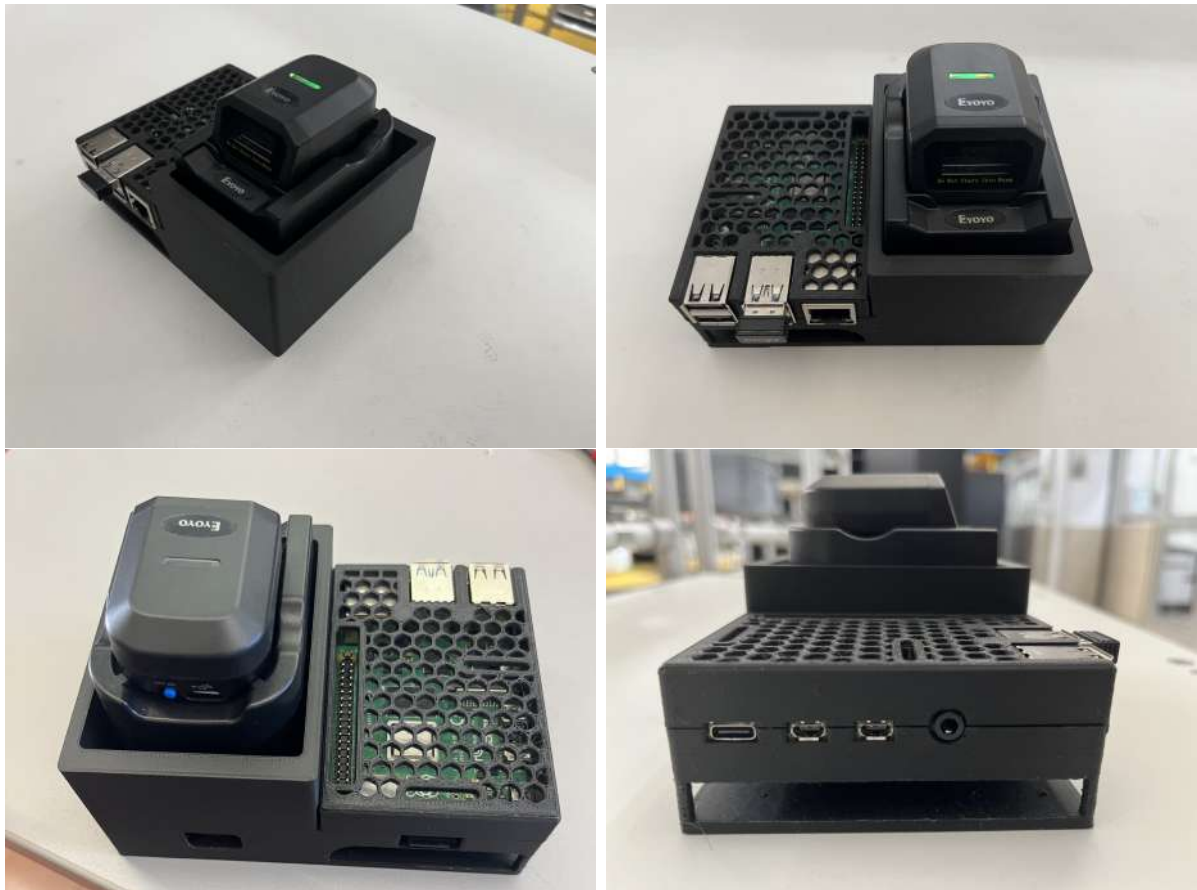
Figure 4.20: Different views of the scanner and Raspberry Pi of one of the workstations in the 3D printed support.
