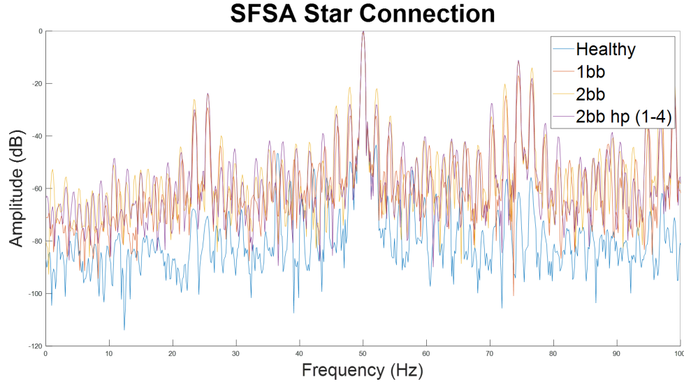
Figure 4.26: Star SFSA results in the different proposed cases: healthy, 1 broken bar, 2 adjacent broken bars and 2 non-adjacent broken bars (1-4)
