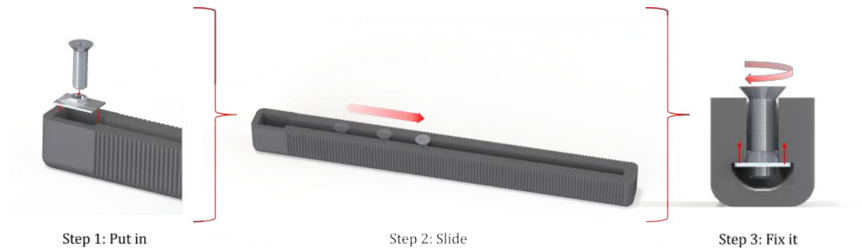
Figure 5.18: Overview of the functionality of tracks
