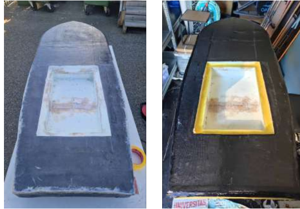
Figure 7.23: Before and after the edges have been filled.
