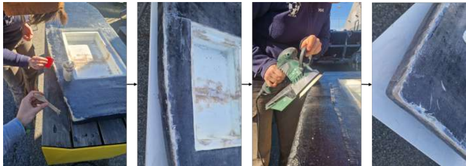
Figure 7.21: Process of filling the edges. It was necessary to make it by hand, and sand it after drying to have an uniform result.
