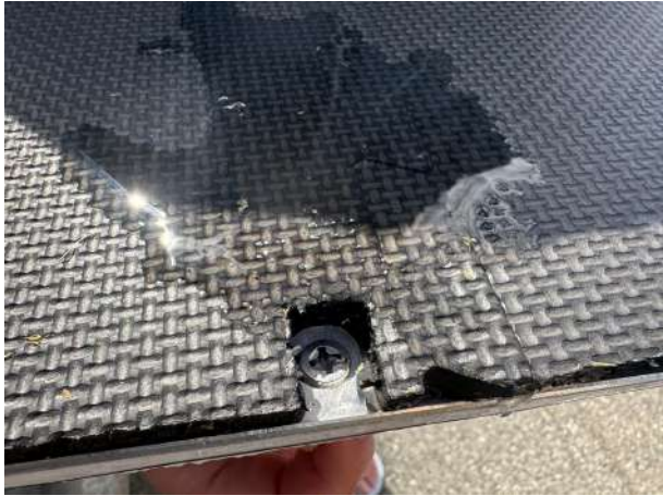
(a) Water in screw hole
