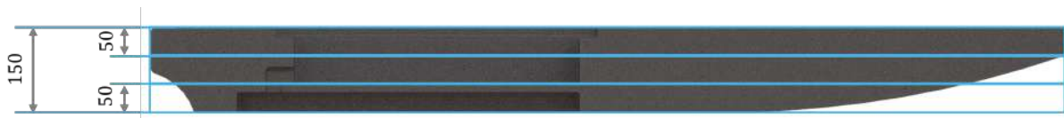
Figure 5.11: Scheme of the cut so it can be possible to be manufactured with the CNC machine.
