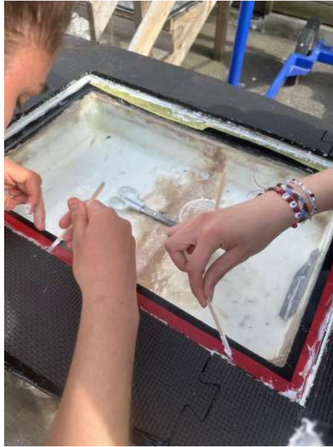
Figure 9.2: Silicon in the gaps between plate and battery case
