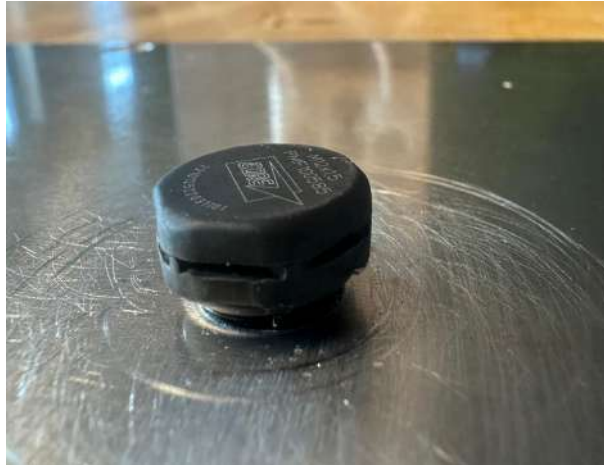
Figure 7.25: Ventilation system assembled to the cover
