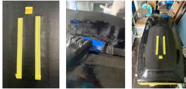
Figure 7.19: Process for final glazing since protecting the tracks with masking tape until afteran uniform distribution have the final result.
