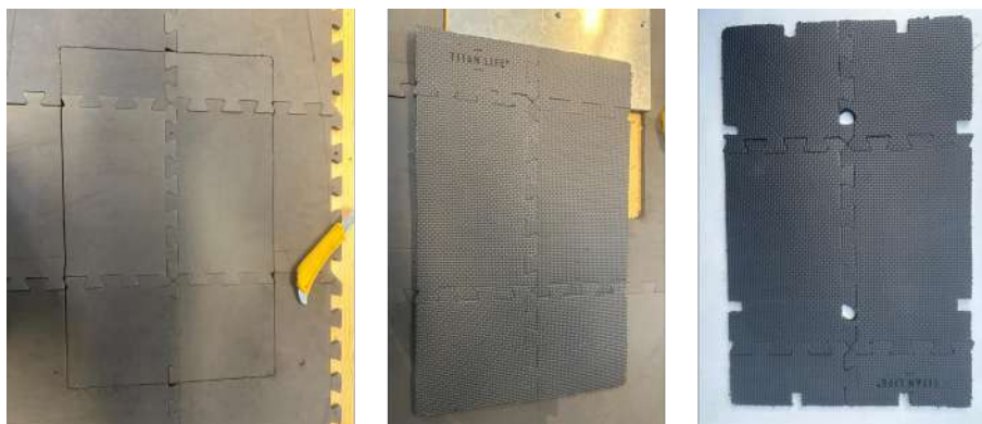
Figure 7.12: Proces of cuting the grip forthe cover since the initial drawing until the screw placement.
