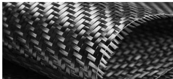
Figure 4.4: carbon fibre reinforced plastic fabric(Innovates, 2025).
