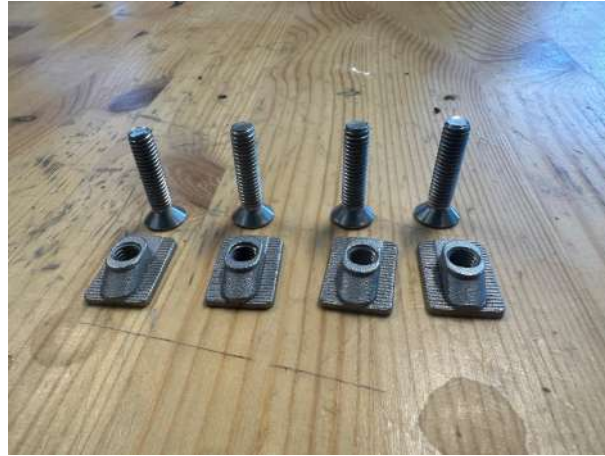
Figure 5.17: Track nuts and screws from the strut base.
