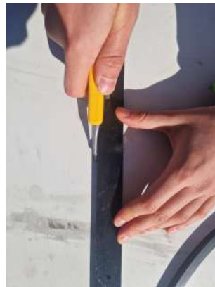
Figure 7.9: Cutting tabs with a cutter knife
