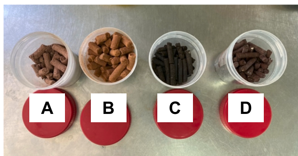
Fig. 2. Packing materials tested in this work. (A) UgnCleanPellets® S.1.0, (B) UgnCleanPellets® S.3.5, (C) pelletised sewage sludge compost (PSS) and (D) pelletised sewage sludge compost doped with Fe salts (PSS-Fe).
