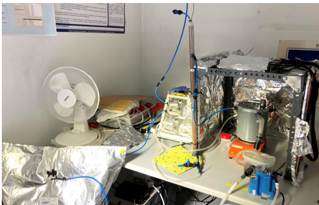
Fig. 3. Experimental set up: (a) schematic reactor configuration and (b) picture of the reactor. 1: gas bag for nitrogen gas, 2: pump, 3: column, 4: tank for influent, 5: reactor, 6: IR light (850 nm), 7: tank for effluent.
