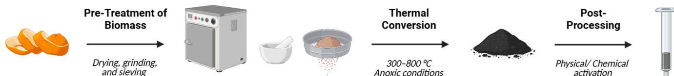
Fig. 3. Main steps in the synthesis and activation of biochar-based sorbents.
