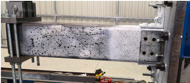
Fig. 4. Column-to-base plate joint with disconnected lateral angle cleats.
