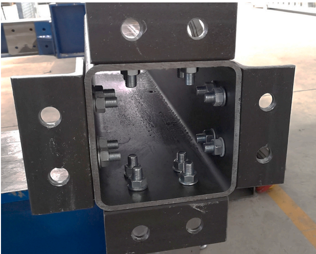
Fig. 2. Interior view of a demountable column-to-base plate joint with bolted angle cleats.
