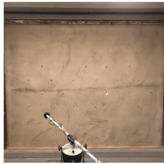
Fig. 3a. Stage 1: The 24 drilled small holes ( \Phi = 1.4 cm).
