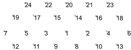
Fig. 3b. Sequence of drilling holes in Stage 1 and opening tabs in Stage 2.
