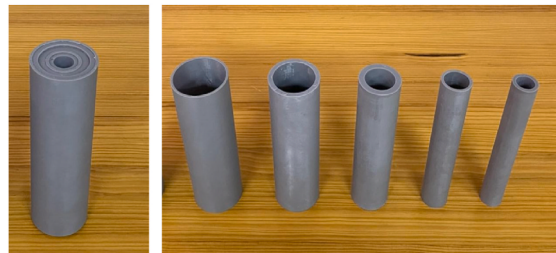
Fig. 6b. Stage 3: 3D-printed resin tubes with diameters from 1.89 to 5.9 cm.
