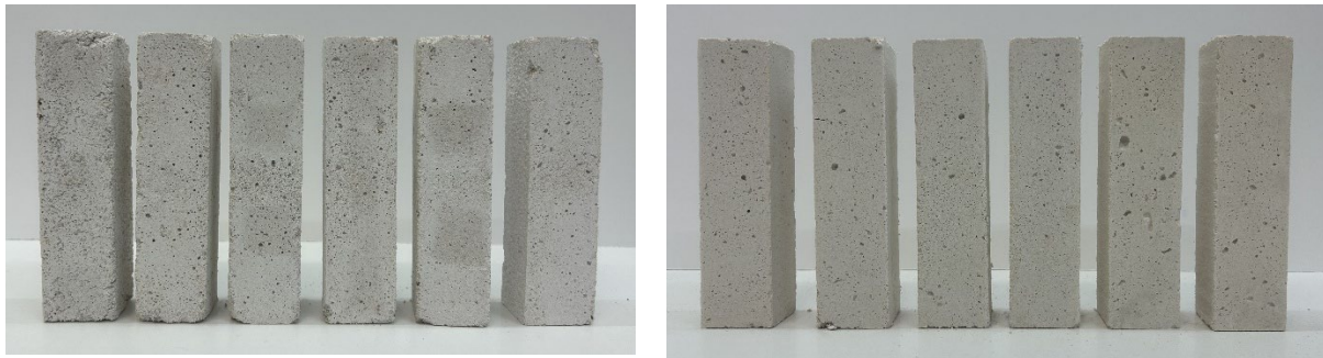
Figure 2. Prismatic mortar samples. On the left, aerial lime samples; on the right, hydraulic lime samples.
