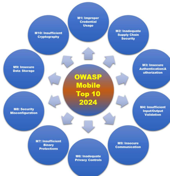
Figura 10. OWASP Mobile Top 10 2024 (M6, M9, M10) [57]
