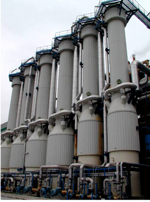
Fig. 2. Six evaporation units for the evaporation section in a beet sugar factory in Spain.
