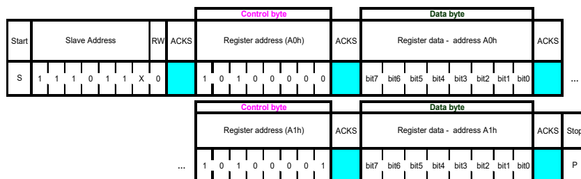
Figure 9: I 2 C multiple byte write (not auto-incremented)
