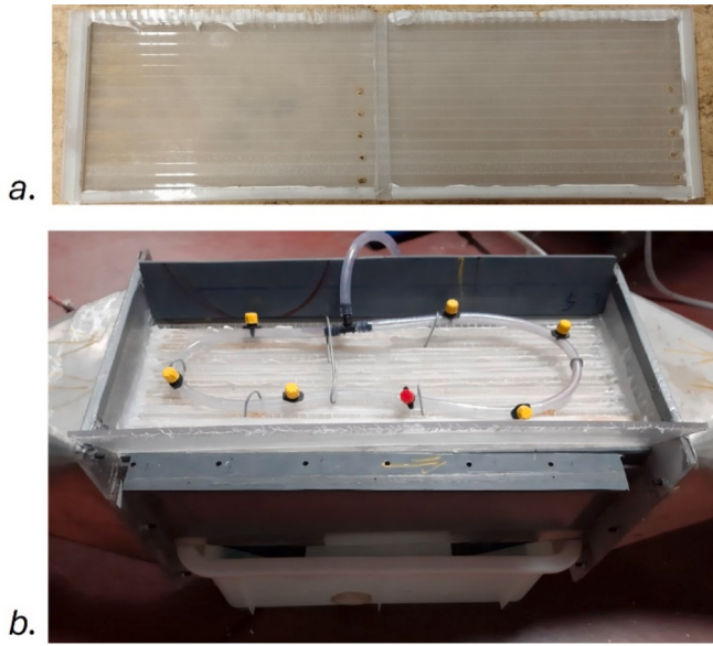
Fig. 2. Actual DPIEC prototype: (a) Detail of one polycarbonate perforated plate and (b) global view of the assembled prototype including the water distribution system.
