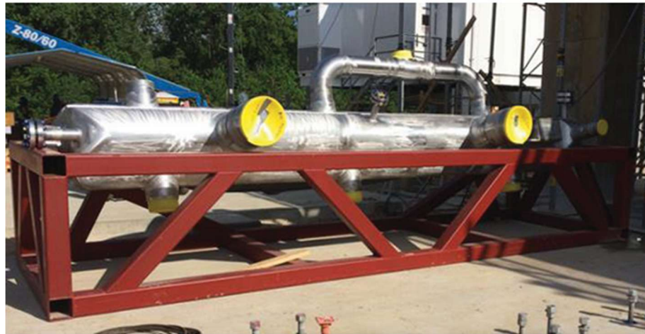
Fig. 2.12. PCHE for the low-temperature section of the RHE of the NET Power cycle demonstration pilot plant.
