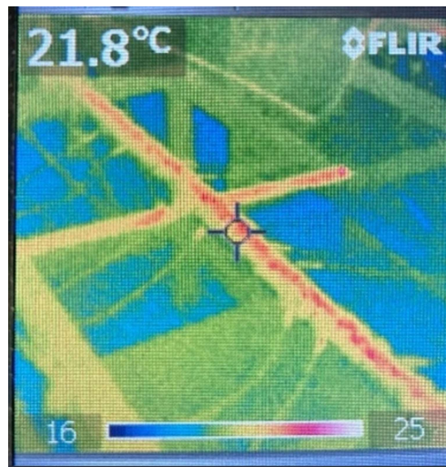
Fig. 5.11. Validation of the thermal insulation by a thermographic camera.
