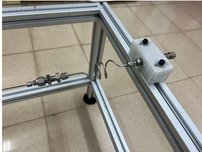
Fig. 5.7. 1/8 " helical tube, used to maintain the test rube straight.
