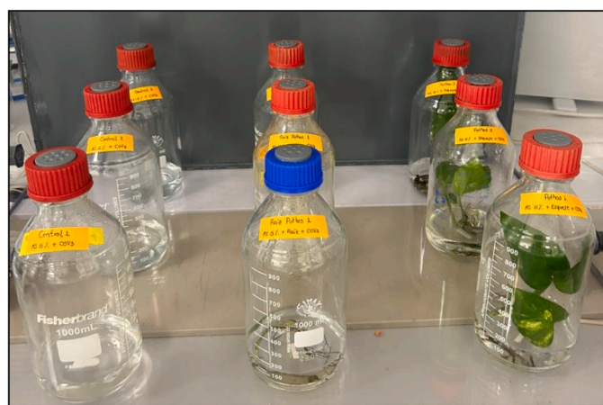
Fig. 2. Experimental setup to assess VOC removal by cuttings in gas-tight bottles.
