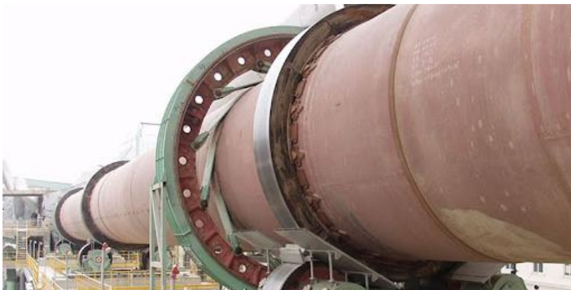
FIG.72: HORNO DE CLINKER http://heavy-plants.com/1-7-rotary-kiln.html
