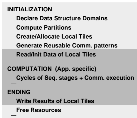
Fig. 2. Typical Hitmap stages for scientific computing applications. Dark grey stages contain sequential code that can be hierarchically parallelized.
