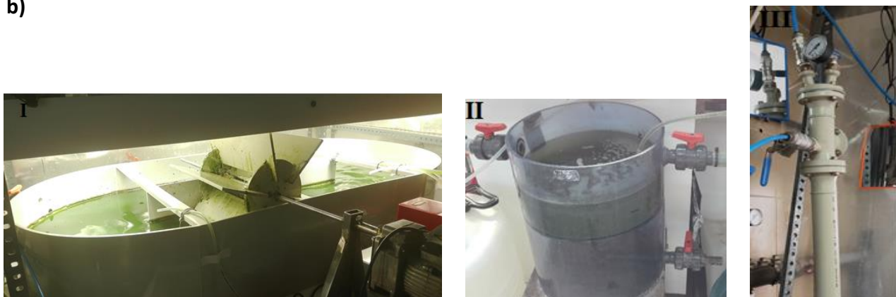
Fig. 1. a) Schematic diagram of the indoor experimental set-up for photosynthetic biogas upgrading and b) photograph of the pilot scale system: I pond, II settler, III biogas scrubbing column.
