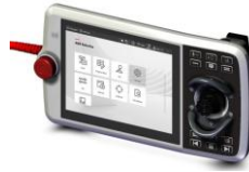
Figura 79. FlexPendant Omnicore (ABB, User manual – FlexPendant, 2024)
