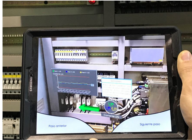
Figure 19: AR guide step-by-step applied to maintenance tasks in the electrical panel.
