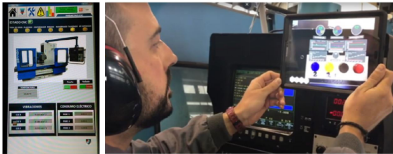
Figure 13: a) CNC's HMI software to interact with the operator. b) Real-time AR app installed on a Samsung tablet.
