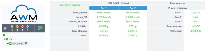
Figure 10: Milling machine dashboard detail in AWM cloud platform.
