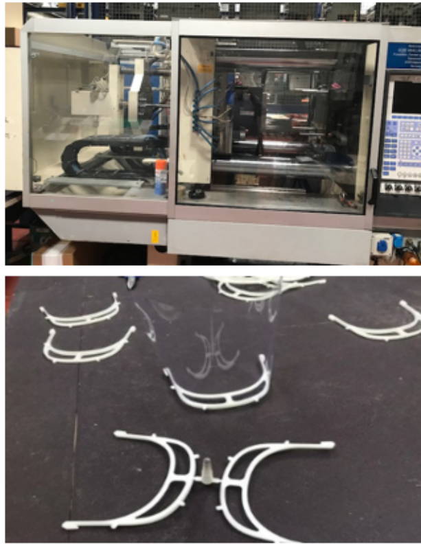
Figure 20: Two-component injection moulding machine Krauss Maffei 200-700 C2 and protective face shields at the R&D facilities.
