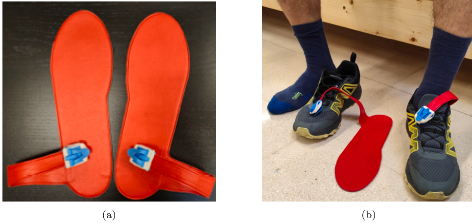
Fig. 3. (a) Loadsol® Instrumented insoles and (b) Example of instrumented insoles usage.
