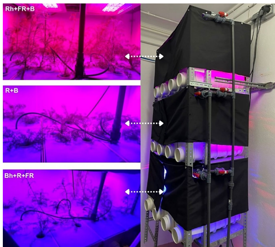
Fig. 1 Aeroponic system with three cultivation trays under different artificial lighting treatments for Matricaria chamomilla : Rh + FR + B (Red predominant + Far-red + Blue), Bh + R + FR (Blue predominant + Red + Far-red), and R + B (Red + Blue)
