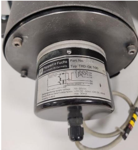
FIGURA 5: ENCODER INCREMENTAL TRD-GK100-RZ
