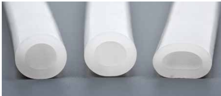
Fluctuations in the extrudate geometry
