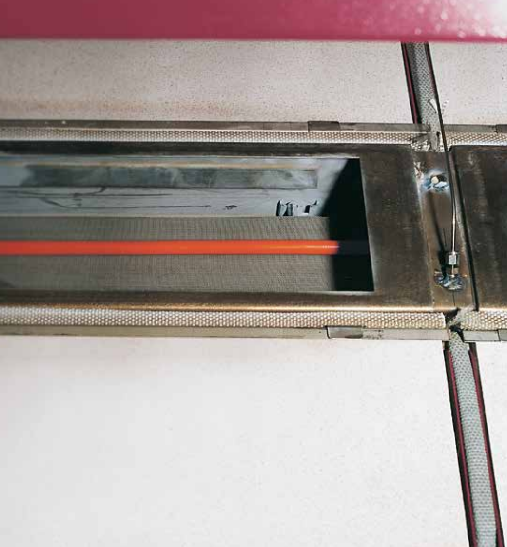
Hose vulcanization in a horizontal hot-air tunnel
