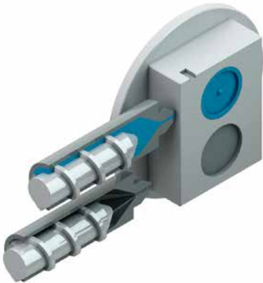
2K injection molding on one injection molding machine
