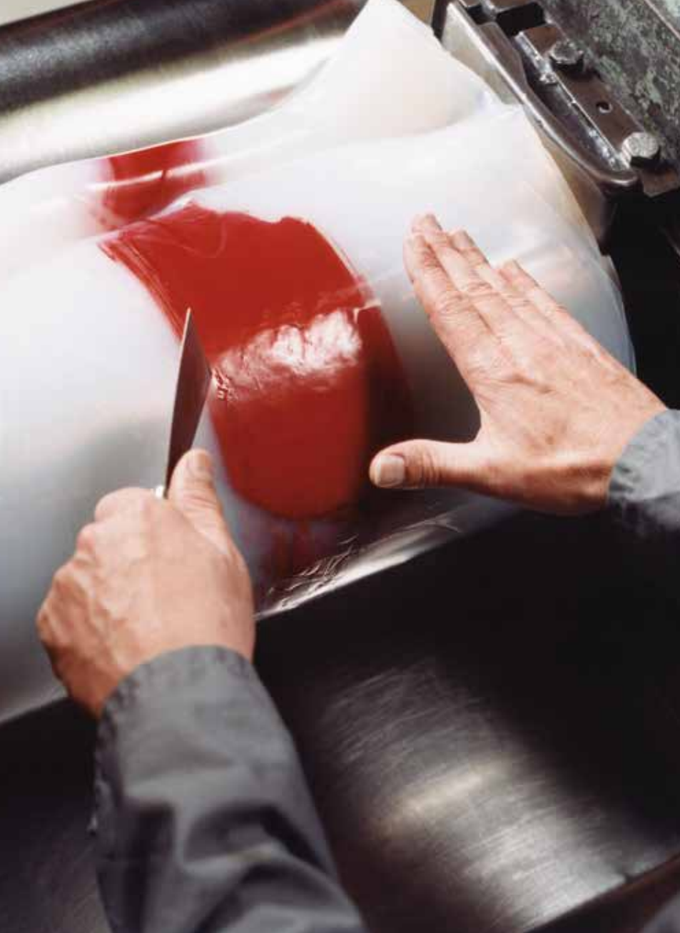
ELASTOSIL® pigment pastes blend especially easily and fast into rubber compounds on the roll mill
