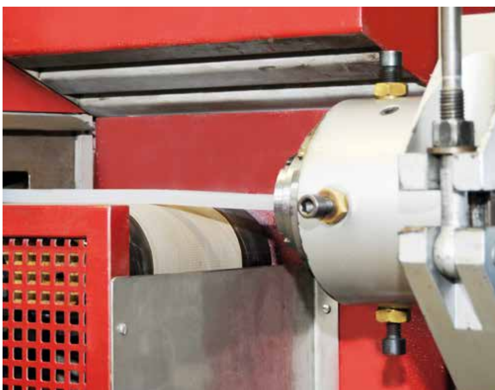
Extrusion of ELASTOSIL® solid silicone rubber into tubing
