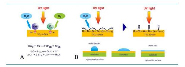
Figure 2.13 .Photocatalytic reaction on TiO₂ surface (Source: Research Centre for Nanosurface Engineering)
