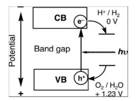
*Figure 2.10. Energetic diagram of a semiconductor during photoexcitation process (Source: Lingsebigler, 1995).*
