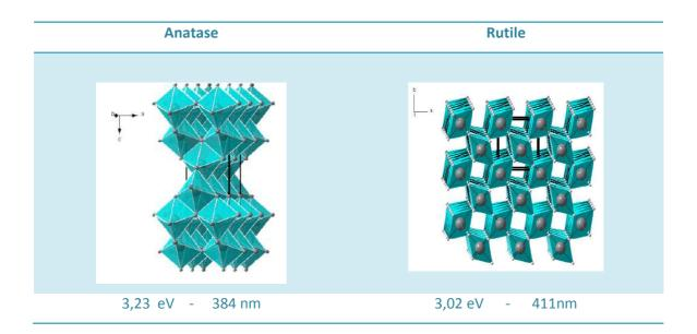
Figure 2.5. Crystal structure of anatase and rutile. (Source: Candal, 2001)
