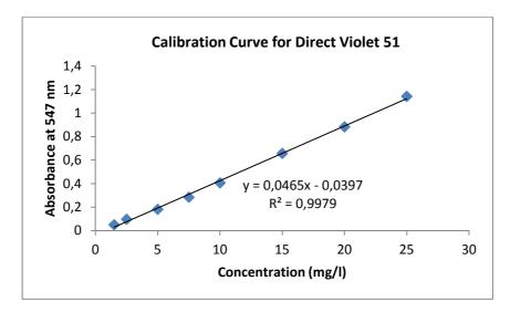
Figure 6.2 . Calibration curve for Direct Violet 51.
