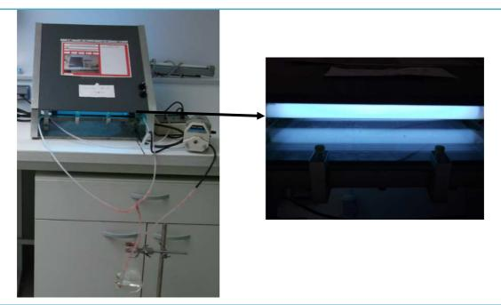
Figure 5.1. Experimental installation of photocatalysis
