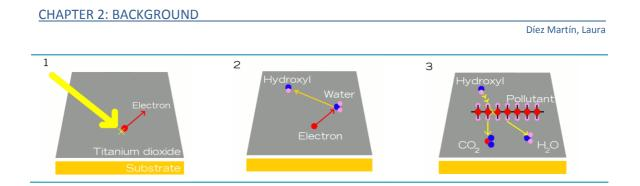
Figure 2.14. Sketch of a photocatalytic process (Source: ExplainThatStuff).
