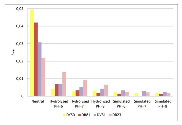
Figure 6.9. Apparent rate constants for dye solutions.
