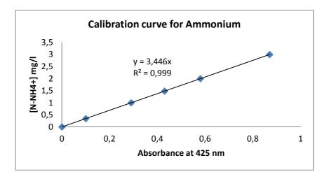
Figure 4.5. Calibration curve for ammonium
