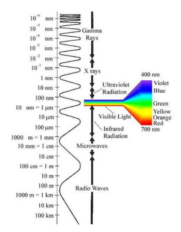
Figure 2.6 . Electromagnetic spectrum (Source: University of Arizona)
