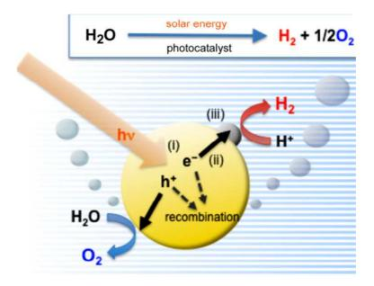
Figure 2.12 . Scheme of heterogeneous photocatalytic process (Source: Solar Energy Materials and Devices Group of Renewable Energy laboratory).
