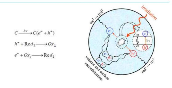
*Figure 2.11. Global reaction in heterogeneous photocatalysis. (Source: Palmisano et al, 2007).*
