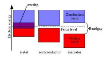
Figure 2.9. Bandgap for metals, semiconductors and insulators.
