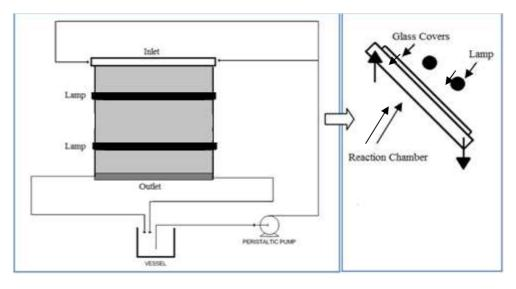
Figure 5.2. Flow diagram of photocatalytic reactor.
