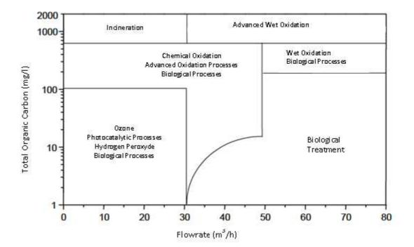
*Figure 2.8. Range of application of AOPs and other treatments (Source: adapted from Forero et al, 2005).*
