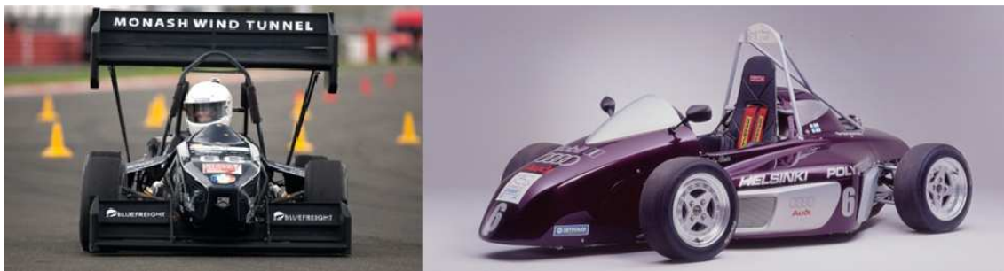
Image 10. Two different concepts for the same competition. High downforce (Left) and low drag design (Right).
