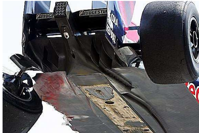
Image 4. Detail of the RB8 rear diffuser. Notice the inlet on the step in order to create a “double diffuser” [29]
