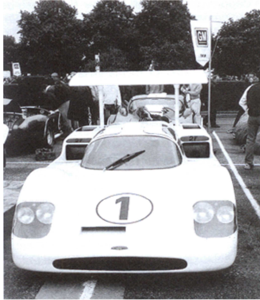
Image 2. Chaparral E2. The first car that competed with an aerodynamic attachment. [27]
