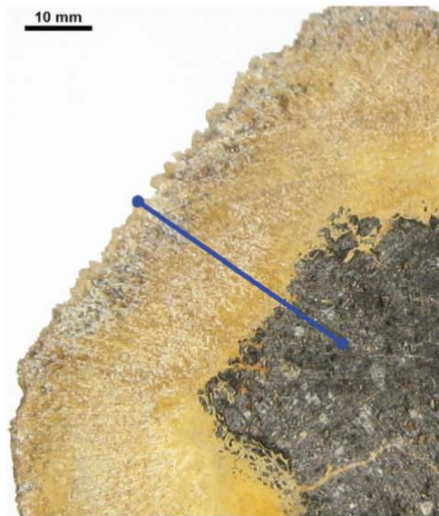
Fig. 3. Flat surface of a carbonate cement extracted from a volcanic breccia in Svalbard (Norway). The inner part consists of a basaltic core (black), cemented with Mg-Ca carbonates (orange).
