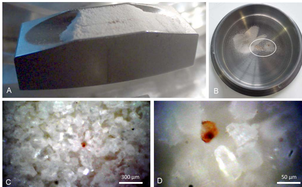
Figure 4-24. Cross-contamination on the calcite 45-125 microns simple. Flattened surface (A), rest of sample in the funnel after dosing with reddish features (B), MicrOmega emulator camera (C) and RLS images (D). The red features are iron oxides.
