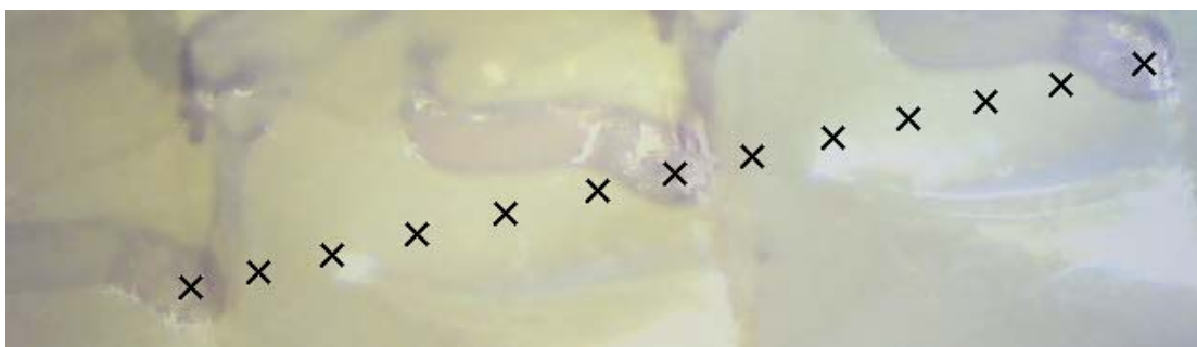
Figure 4-8. Reference for the calibration of the RLS spot path under the MicrOmega emulator FoV.
