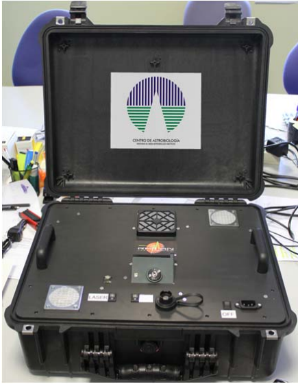
Figure 2-28. Integration the RAD1 spectrometer in a field setup
