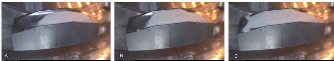
Figure 4-12. Sample surface after the first (A), second (B) and third (C) dosing and flattening steps for the gypsum 45-125 \mu\text{m} sample.
